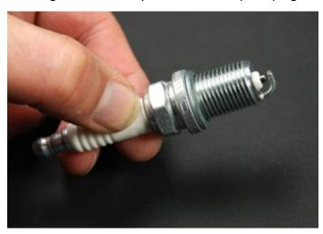
start; no spark, no start. Spark plugs wear out. They often need replacing due to using stale fuel in your mower. Blocked air filters and oil filters can affect the performance of the spark plug. It is wise to replace the spark plug as a matter of course every season. On most mowers, it is not a difficult job. You just need the right tool to grab on to the plug to twist it out of its socket. Not all spark plugs are alike so check the owner's manual for the plug specs for your mower.
