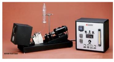
the end of the test, the heater is turned off and the panel is allowed to cool. Once cooled, the test panel is removed, washed with solvent to remove any excess lubricant, and weighed to determine the amount of deposits adhering to the surface of the panel. The darker the color of the panel, the more deposits that have been left. A cleaner panel indicates fewer deposits.
