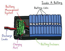
too low), over-current (if the current is too high during charge or discharge) and short circuits. It often can help prevent discharge if the temperature is too high or low, and can also help balance the cells to ensure they all stay at the roughly the same voltage during charging.
