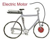
We mostly sell hub motor conversion kits where the motor is built inside the bike wheel and the axle of the motor is secured in the bicycle dropouts. The axle is fixed to the bicycle fork and then when you provide power to the motor the "rotor" part of the motor spins, which then spins the bicycle wheel itself.
