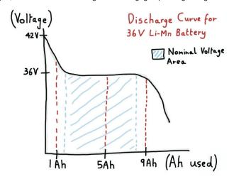
For example, a 36V Lithium Manganese (LiMn) battery is 42V when hot off the charger, whilst it will tend to operate around 36-38V for most of the discharge. A 48V Lithium Iron Phosphate (LiFePO4) can be as high as 60V at the end of charging but will normally operate around 48-52V whilst discharging.
