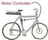
The motor controller delivers and regulates power to the motor, controls how fast the motor spins (via a throttle normally) and converts the DC (direct current) type of electricity the battery provides into the AC (alternating current) electricity needed to spin the hub.
