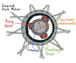
Geared hubs have a high RPM motor inside with a planetary transmission linking it to the low speed of the bike wheel. They also have a built-in freewheel that disengages the motor so that the wheel spins freely with no drag when not in use. Together these make for a lighter hub motor and a ride experience that is closer to a normal bike, but because of the freewheel they cannot do regenerative braking.
