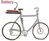
The battery is where the system gets its power from. Nowadays most ebike batteries are lithium batteries, similar to those found in laptops but are about 10x the size. The battery is usually recharged by a charger plugged into a mains power outlet. A battery weighing around 4kg can provide upwards of 20-40km range with speeds of 30-40kph depending on how much the rider pedals.
