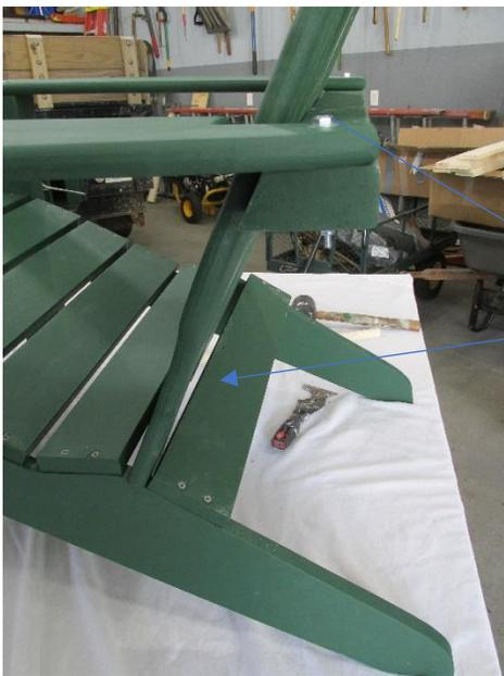
Step H) Place the state back (mitten) of the chair in the opening of the **seat between the 6<sup>th</sup> and 7<sup>th</sup> seat boards.**
