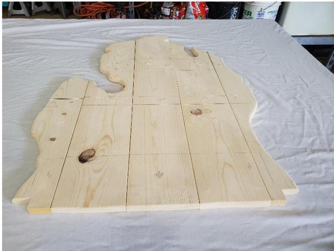
Back Boards laid out showing lines for mounting back supports. Top Brace: 1 x 15" and bottom brace 1 x 19.5; center brace 2x4 with angled edge cut
