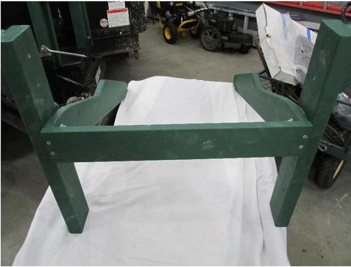
Step C: Assemble the front seat board (Marked FB). **This front seat board takes (4) – 1 5/8" screws.** The front seat board sets the distance of the 2 front legs. It sits between the 2 legs and mounts flush to the front ends of the leg/seat board support. You may wish to pre-drill holes into the ends of the leg/seat boards. The front seat board (FB) is considered board #1 of the 7 seat boards.
