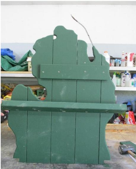
Step G) Align state back boards with pencil side up. If you have painted your boards, the top brace (TB) lower edge will be placed 21" from the bottom edge. Secure with (4) 1 1/4" screws. Place the center brace (CB) lower edge at 12" from the edge. The sides of the 2x4 Center Brace should be 1 3/4" over on each side of the back of the chair. When aligned, screw in (5) 1 1/4" screws.
