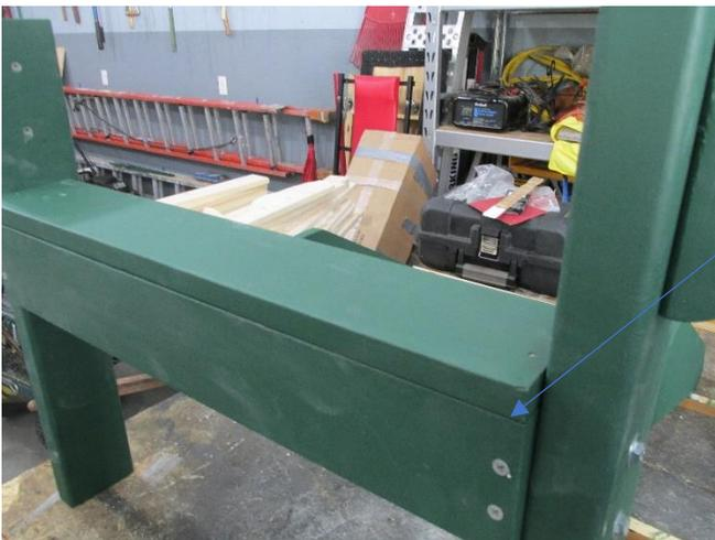
Step D) Place seat board #2 at the front edge of the front board (FB). Screw in using 1 1/4" screws
