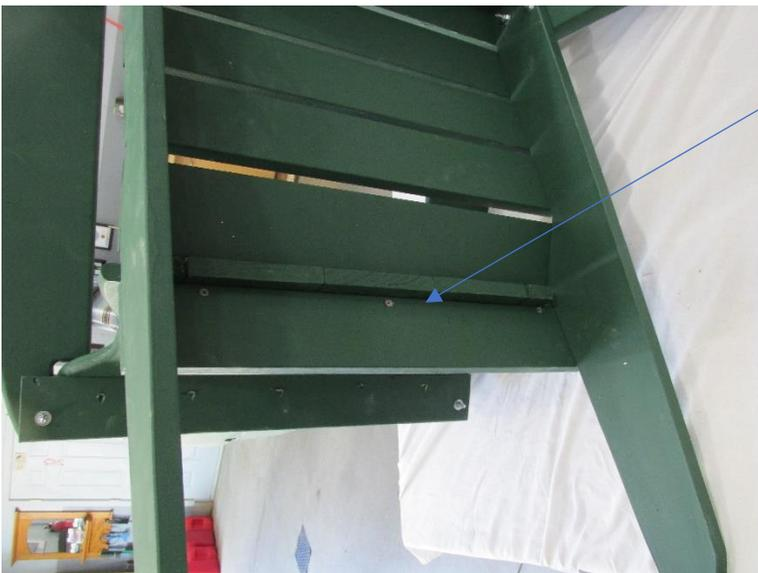
Step K) Tip the chair over and secure the state back and (BB) to the 7<sup>th</sup> board using (3) 1-5/8" Philips screws.
