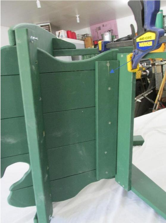
Step J) Secure the bottom brace (BB) with (5) 1 1/4" screws.
