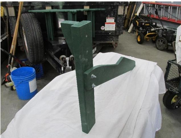
Step B) Assemble the front legs (Step A) to the leg/seat boards with (2) bolts, (2) nuts and (4) Washers on each leg. You will need to be on level ground. This picture is of the left front leg. You will have a similar assembly for the right front leg.
