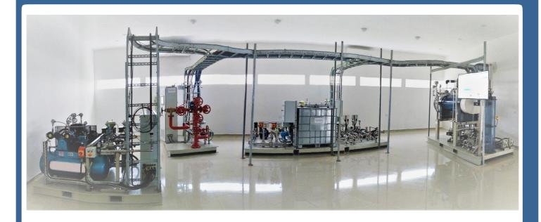
Multiple training outcomes Operates as an integrated plant or individual stand-alone trainers DCS / PLC control options Large screen display and local HMI visualization & control
