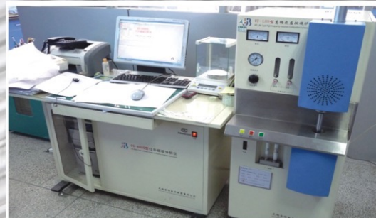
GS-8800型红外碳硫分析仪 GS-8800 Type Infrared Carbon & Sulphur Analysis Instrument
