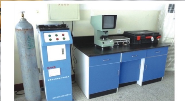
金属撞击试样缺口自动拉床 Notch Bracing Machine for Metallic Impact Specimen
