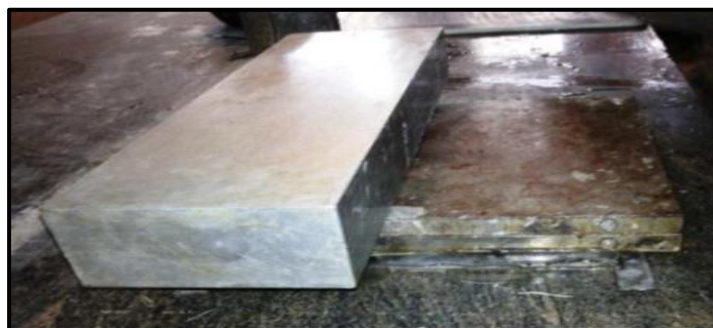
Fig.1.2: Applying Weights on Fabricated Surface
