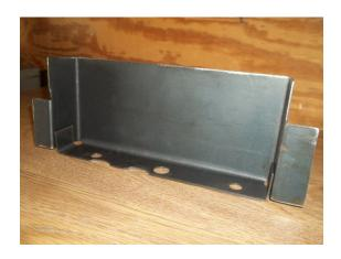
The lower inter strut plate will match the holes in the bottom of the rails. They will match the holes for the K member when installed, be sure measurement are correct. Crush tubes are tacked over the holes to prevent crushing the upper strut plate when tightening. I extended the lower strut plate to allow a good backing to the strut tower skirt as they seem to rust out bad. All the piece can be trimmed to fit your application, crush tubes also may need to be trimmed to fit.
