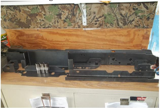
This is a guide for the installation of the Left or Right replacement frame rail. This replacement will require that the engine be removed and all wires hoses or mounting hardware will need to be removed from frame. Radiator will also need to be removed to access the support that the front of the frame rails attach to. Once the frame rails in the car are clear it's time to start measuring.
