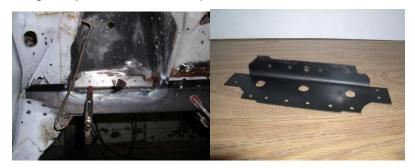
The bottom plate with the three large holes is to weld the crush tubes onto. Check the plate in the rail to be sure the holes line up for the k-member support bolts and now that you know what side
