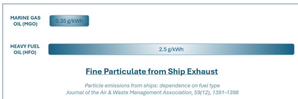
Comparison of Heavy Fuel Oil (HFO) to cleaner Marine Gas Oil (MGO)
