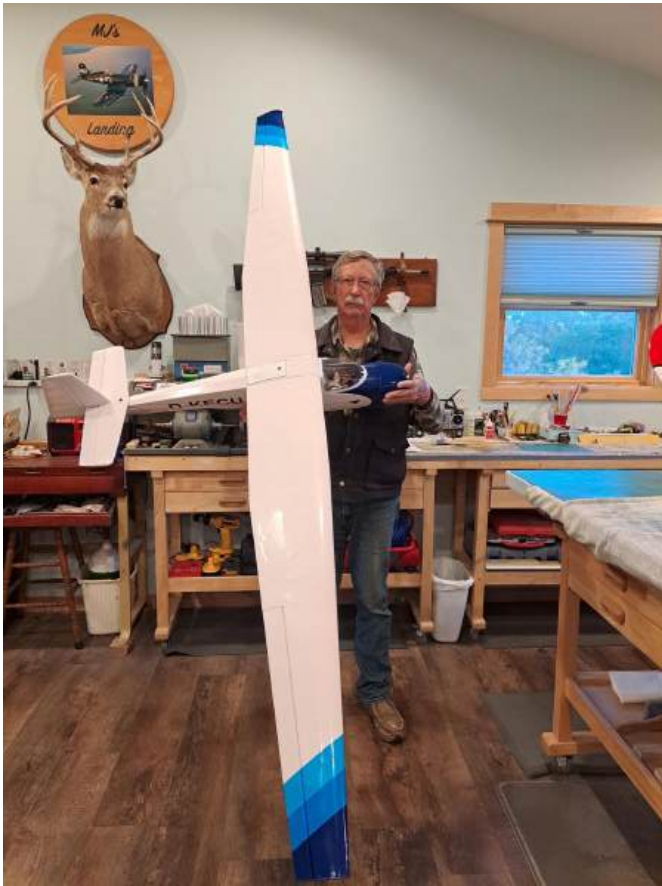
A Newsletter is not complete without another beauty from Mike M's Skunkworks.... 100" Motorspatz post WW2 German motorized glider - Balsa and plywood construction
