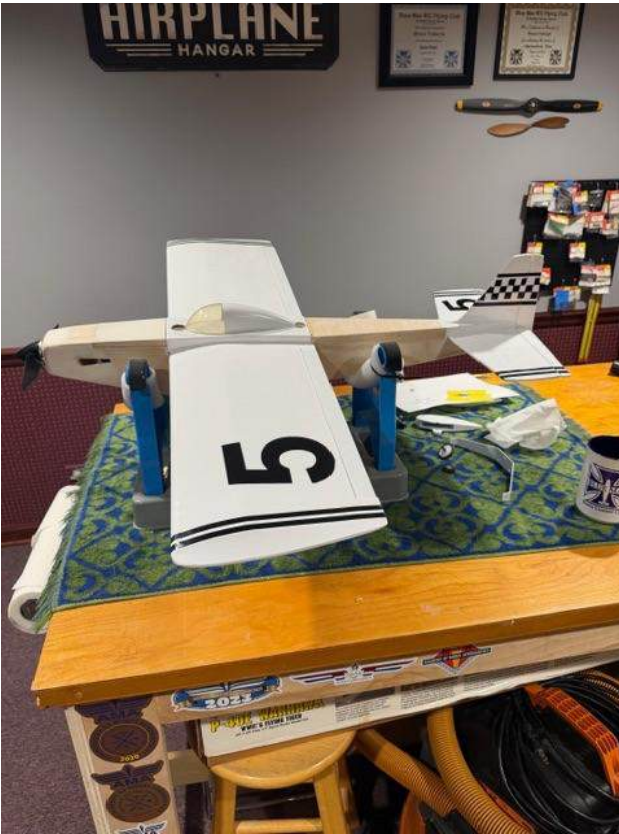
Mike M. Skunkworks... Finished 2nd project of 2026, 22 yr.old GP 1/4 scale Shoestring ARF. Makes me remember why I loathe Monocote ! Saito 100, Futaba FASST, 2000mah 6v. NIMH. Favorite civilian plane.
