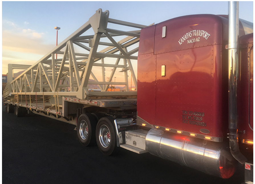
This photo was shot in Bisbee in late October. The conveyor housing for FMI's big new Lone Star project at Safford is being fabricated at Prometal 's facility in Hermosillo and shipped across the border at Naco on its way to Safford. Hundreds of these sections are crossing for the conveyor that will haul Lone Star ore down to the existing SX/EW facilities at the Safford mine. Prometal has worked on a number of projects for Freeport and other mines in the region.
