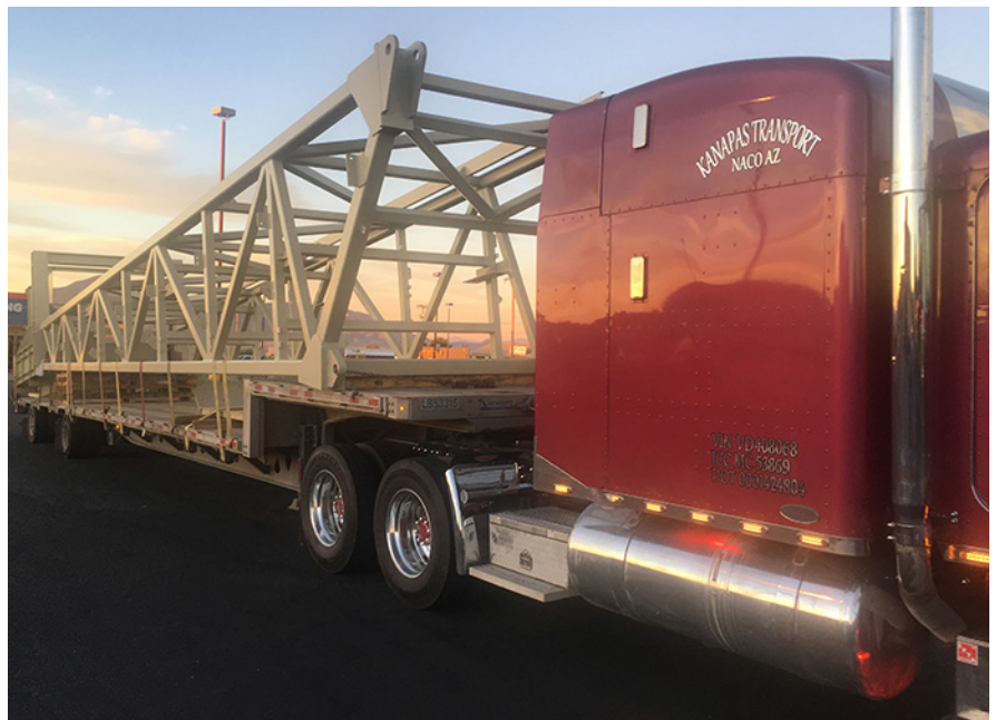
This photo was shot in Bisbee in late October. The conveyor housing for FMI's big new Lone Star project at Safford is being fabricated at Prometal 's facility in Hermosillo and shipped across the border at Naco on its way to Safford. Hundreds of these sections are crossing for the conveyor that will haul Lone Star ore down to the existing SX/EW facilities at the Safford mine. Prometal has worked on a number of projects for Freeport and other mines in the region.
