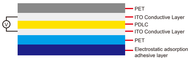
SFB SELF-ADHESIVE PNLC FILM STRUCTURE
