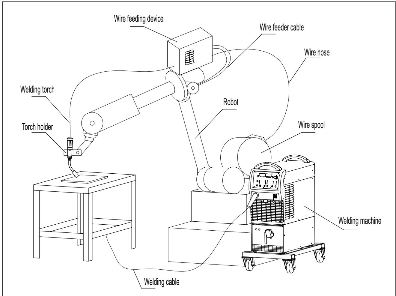
Fig. 4-1-1: System components
