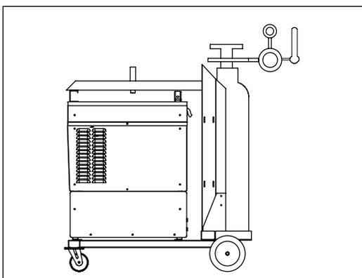
Fig. 4-9-2: Gas cylinder installation
