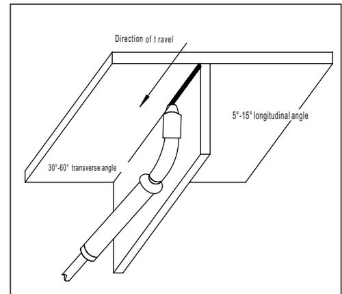
Fig. 7-1-7: Overhead weld
