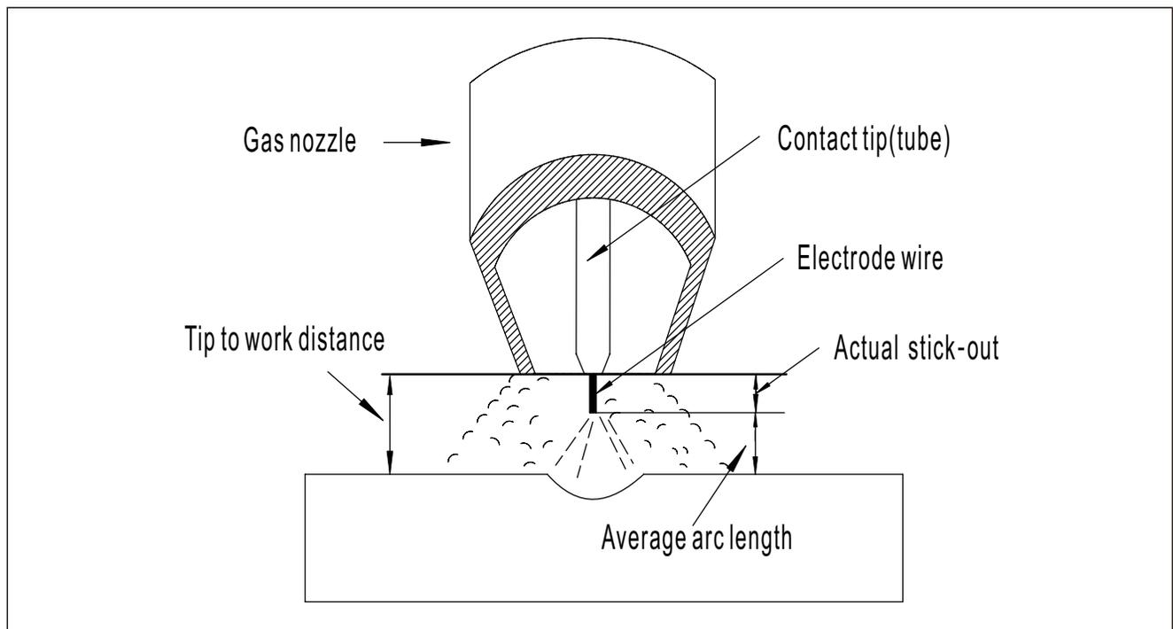
Fig. 7-1-8: Electrode stick-out
