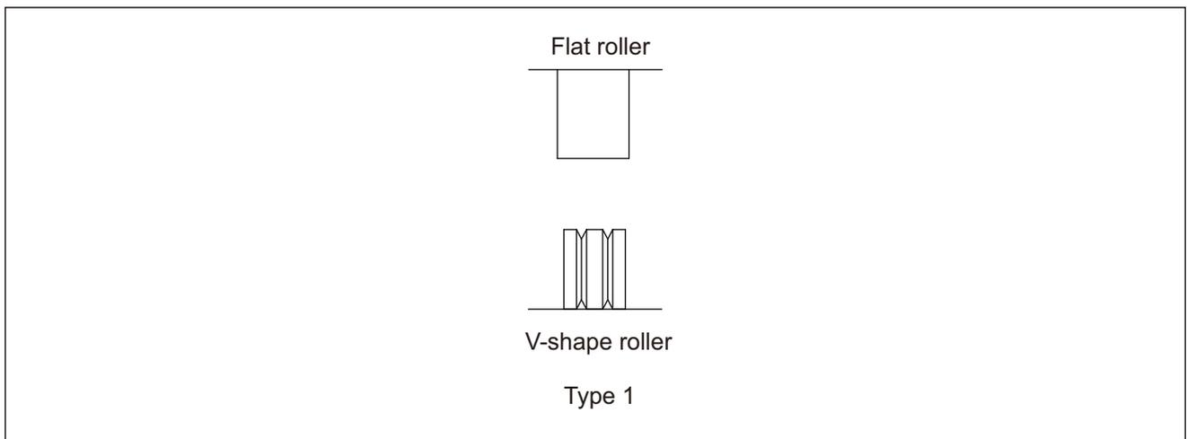
Fig. 4-9-4: Wire feeding rollers
