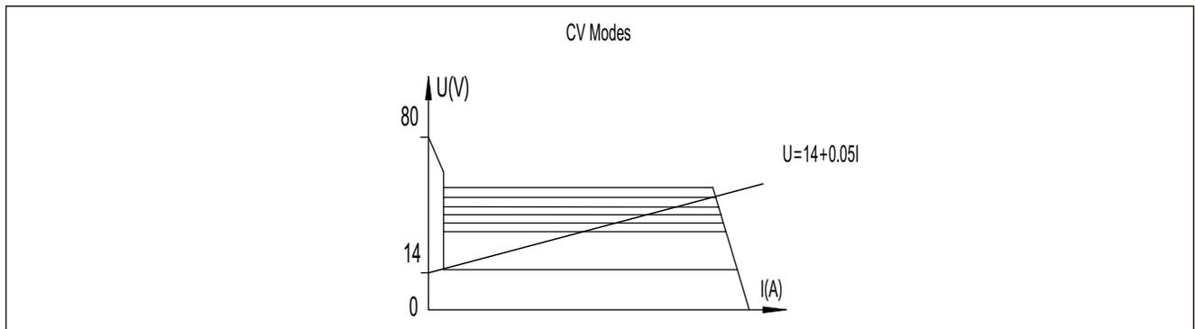
Fig. 1-3-1: Output characteristics
