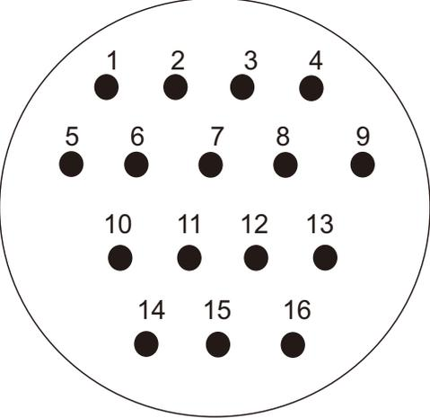
Table 4-4-3: Wire feeder control socket X7
