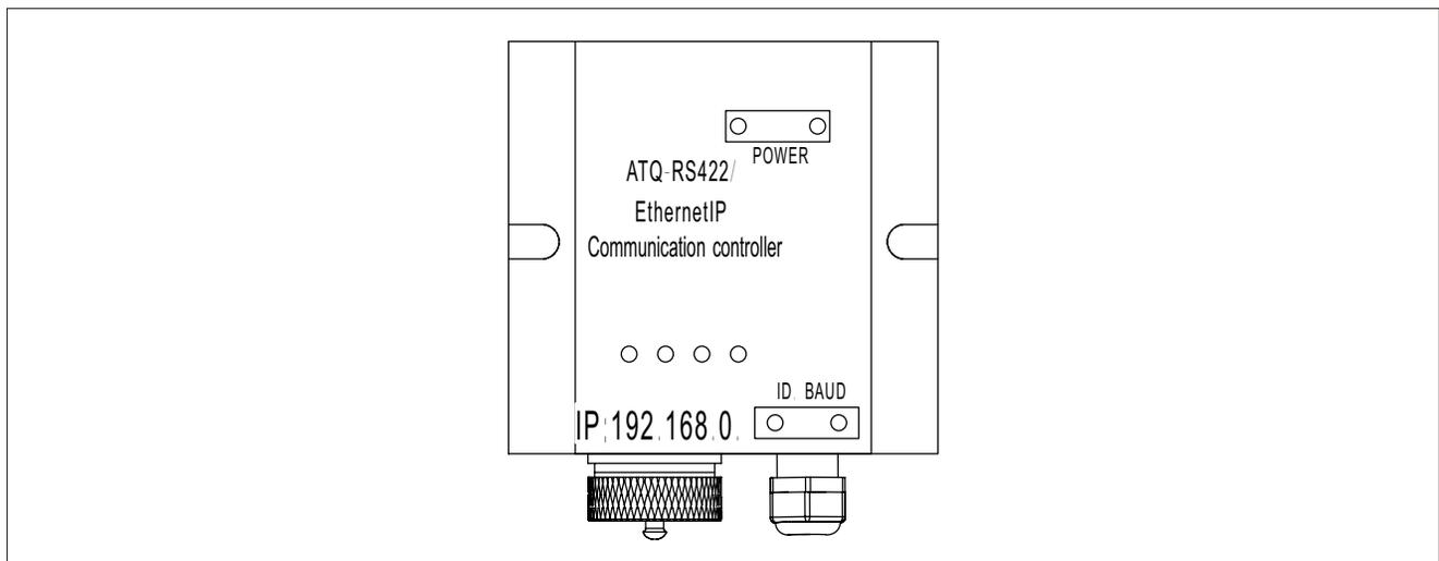
Fig. 4-7-3-1: ATQ-RS422/EtherNetIP interface box
