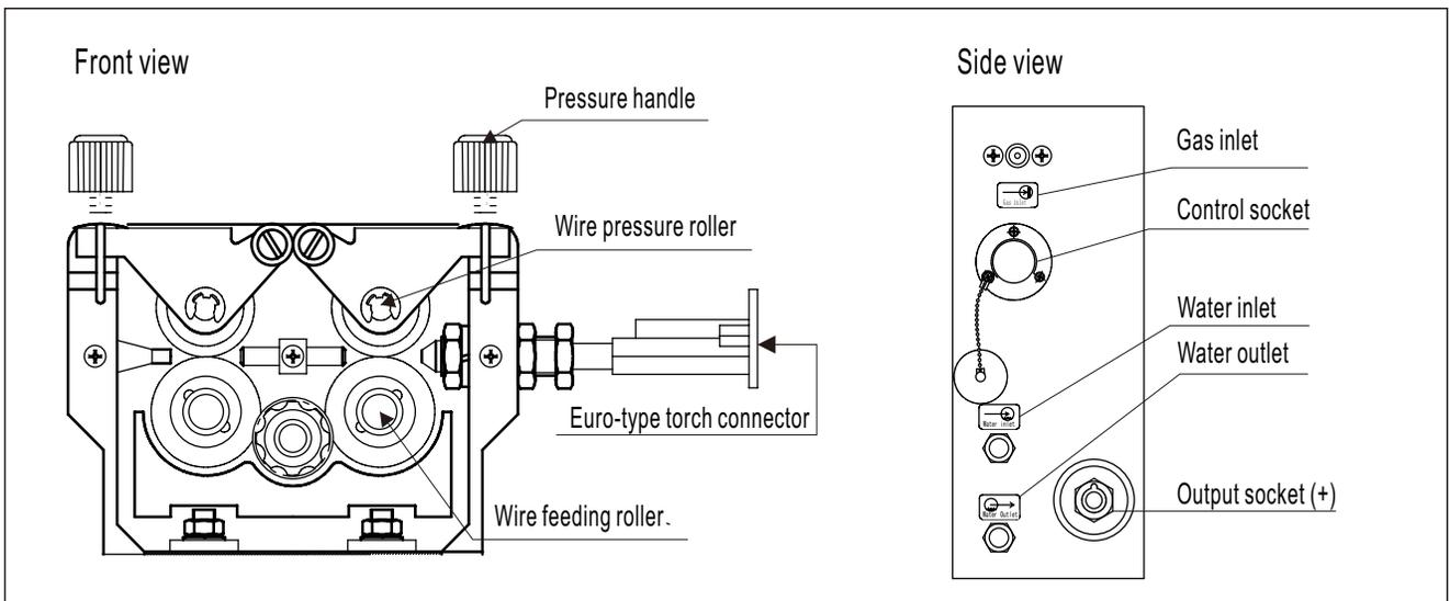
Fig. 4-5-2: Wire feeding device interface
