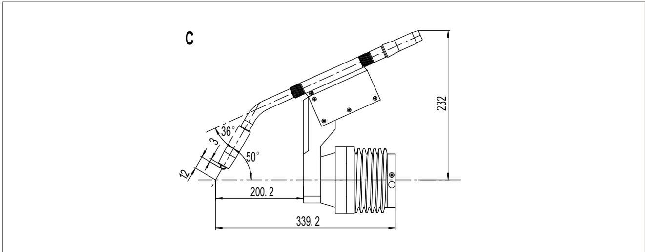
Fig. 4-6-2: Different buckling angle for robot torch neck
