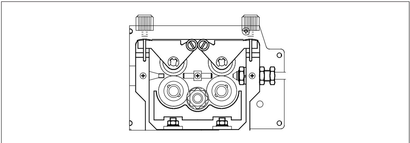
Fig. 4-5-1: Wire feeding device
