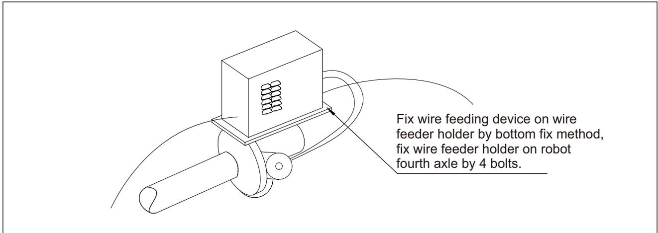
Fig. 4-9-3: Installation for wire feeding device
