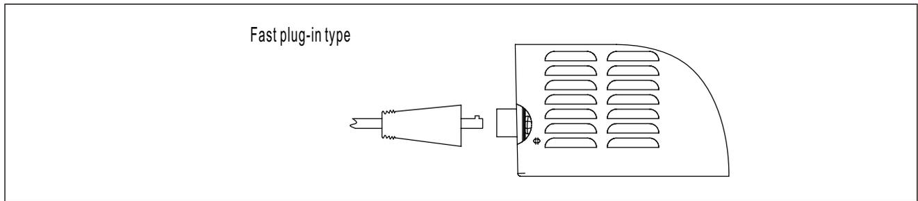
Fig. 4-4-3: Output socket
