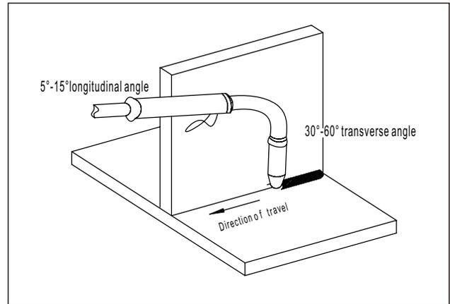
Fig. 7-1-5: Horizontal fillet weld
