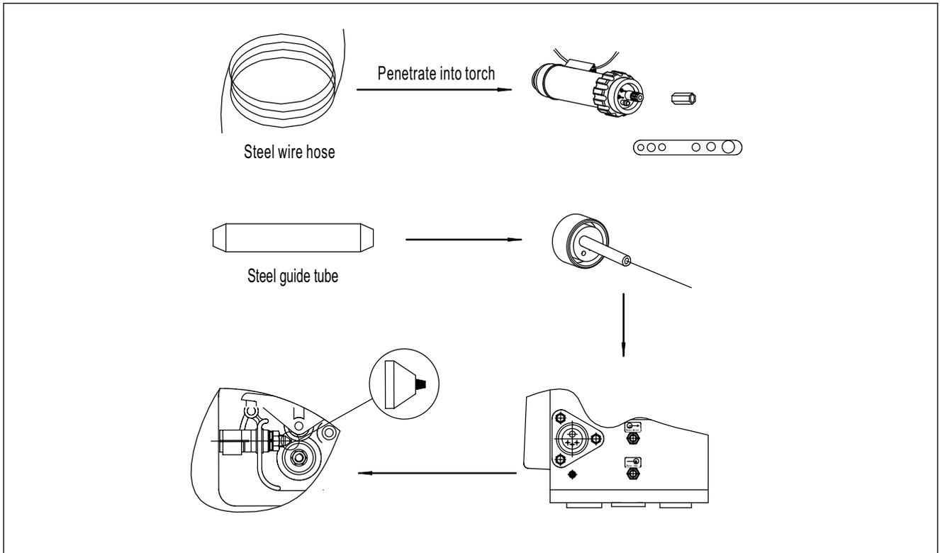
Fig. 4-9-9: Installation of steel wire hose
