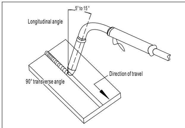
Fig. 7-1-4: Butt & horizontal welds
