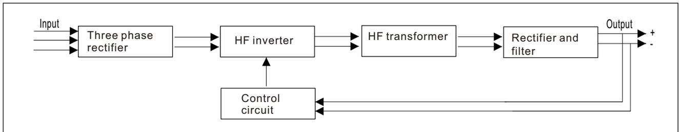
Fig. 1-2-1: Schematic diagram
