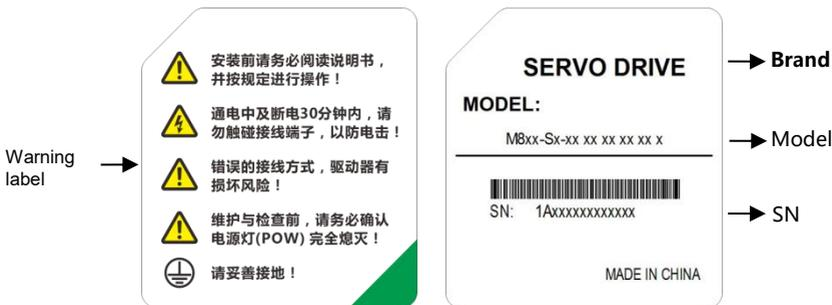
Figure 2-2 Label description of servo drive body
