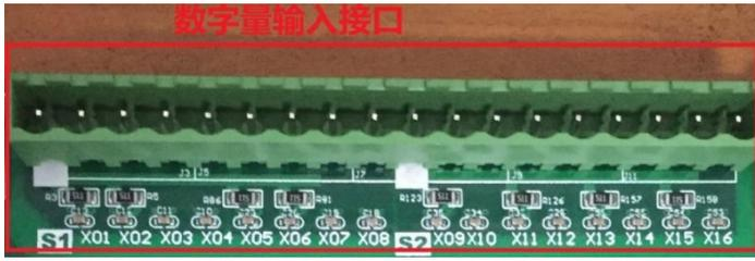
As shown in the figure, the input is divided into two types: X01~X08 with common terminal S1 As a group, X09~X16 with public terminal S2 as a group.
