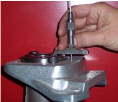
Measure the height of the installed bearing in the axle housing with caliper bracket bolted in position. (Figure # 2)
