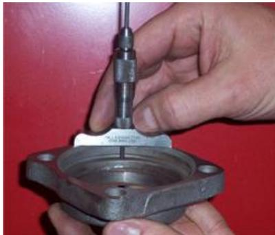
Measure bearing retainer depth. (Figure # 3)
