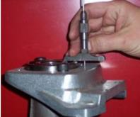
Measure the height of the installed bearing in the axle housing with caliper bracket bolted in position. (Figure # 2)
