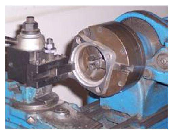
The objective is to establish bearing float (bearing height smaller than retainer depth) of .005" minimum to.010" maximum. This will minimize rotor float and still maintain a good compression of the caliper bracket. For machining, we use a lathe to trim the flange end of the retainer. (Figure # 4) Never attempt to grind this adjustment with hand held grinder.
