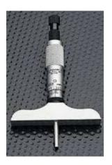
Measurements are observed with a depth micrometer (Figure # 1).
