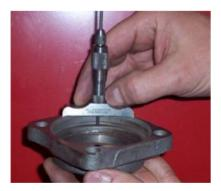
Measure bearing retainer depth. (Figure # 3)
