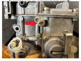
3) There is a very, very small hole in the end of that fitting. Spray carb cleaner through the hole to make sure it is open. If nothing goes through use a very fine wire to dislodge what's stuck in there followed up by another spray with carb cleaner.
