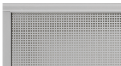
PERFORATED ALUMINUM 0.312" square perforations on 1/2" centers
