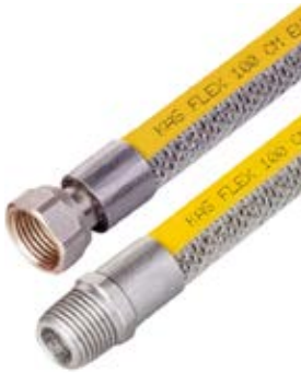
GEFLOCHTENER ERDGAS-ANSCHLUSS FLEXI-MUTTER-NIPPEL / BRAIDED NATURAL GAS CONNECTION FLEXI NUT NIPPLE / ÖRGÜLÜ DOĞALGAZ BAĞLANTI FLEXİ SOMUN NİPEL 1/2"-1/2"
