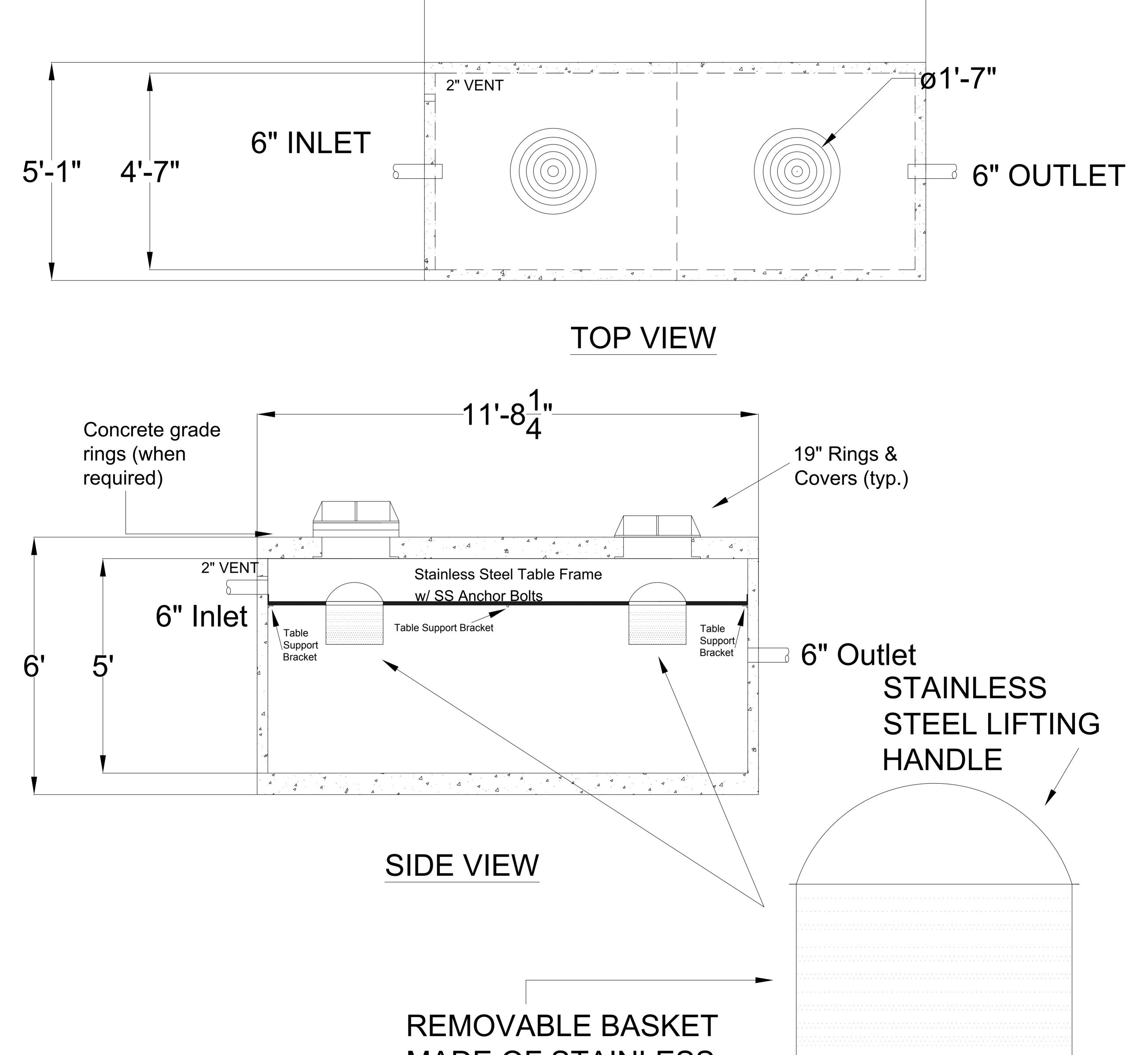
MADE OF STAINLESS STEEL PERFORATED SCREEN w/3/16" HOLES
