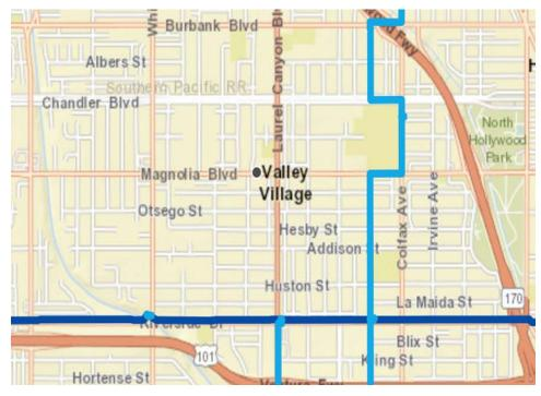
Pipelines and High Pressure (greater than 60 pounds per square inch) Gas Distribution Mains. Lower pressure distribution mains and smaller service lines connected to the gas meters at homes and businesses are not shown here. The lighter blue/grey lines are those that run behind Colfax Elementary and in front of North Hollywood High School (NHHS).
