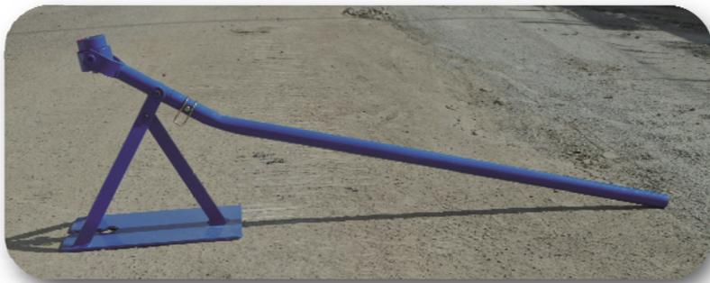
The lever arm increases the extraction force. It can be removed from the tripod to facilitate transport or storage. Jaw can also be removed from the tripod. Ball-bearings are interchangeable in case of wear.
