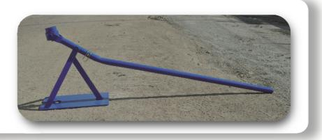
The lever arm increases the extraction force. It can be removed from the triped to facilitate
