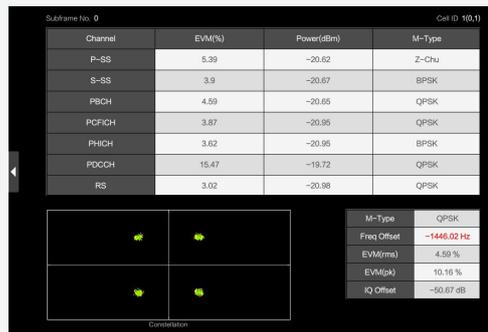
LTE/LTE-A control channel measurement
