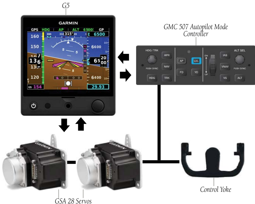
Figure 3-2 Core GFC 500 System
