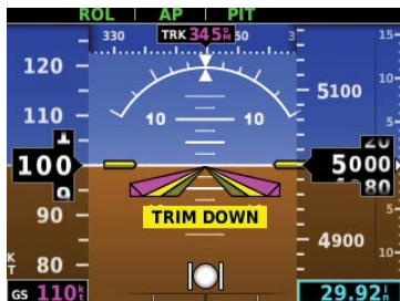
Figure 3-22 TRIM DOWN Alert
