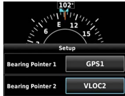
Figure 2-19 Bearing Pointer Setting
