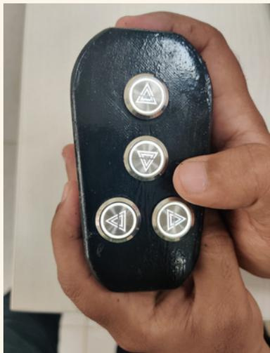
**Press remote buttons 4 times for forward/backward, IN/OUT movement**
