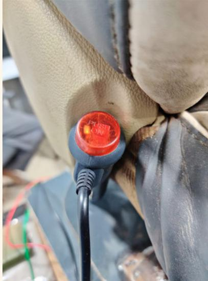
**Press the red button ON for the sensors and electronics. It's near your seat belt clips.**
