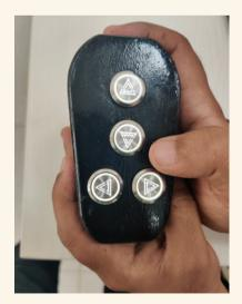
Press remote buttons 4 times for forward/backword, IN/OUT movement
