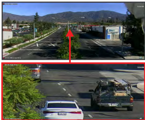
Pan-Tilt-Zoom cameras can read license plates from up to 2 blocks or 200 yards away.
