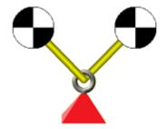
A load-distributing anchor system can be built using rope or webbing. If rope is used, a two-loop figure 8 on a bight with unequal loops can be used. As shown in the illustration on the next page, the rope in the larger loop, between anchor points, is connected to the
