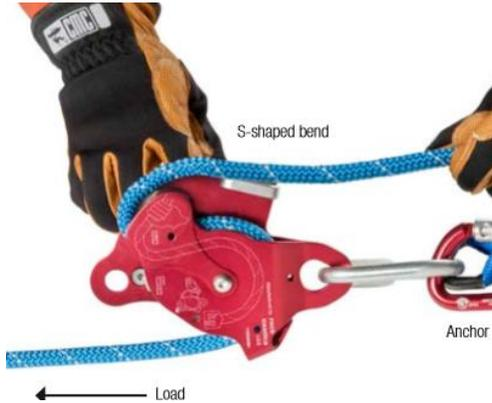
**ALWAYS MAINTAIN A FIRM GRIP ON THE RUNNING END OF THE ROPE DIRECTED BACK TOWARD THE ANCHOR IN AN “S-SHAPED” BEND BEFORE ENGAGING THE RELEASE HANDLE.**
