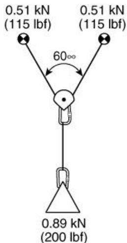
At a 60-degree angle, the load on each anchor will be 50% - 55 %
