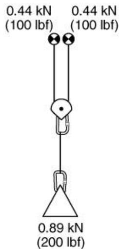
At a 0 degree angle, the load on each anchor will be 50%. With a two-point load-distributing anchor system holding a load of 200 pounds, each anchor holds approximately 50% of the load, or 100 pounds.
