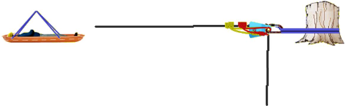
If the FIRST moving pulley in the system is at the LOAD, the system will be odd. This is a 3:1 Mechanical Advantage.
