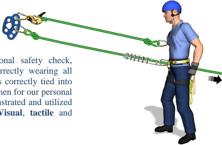
The rescuer being correctly connected into the system.
