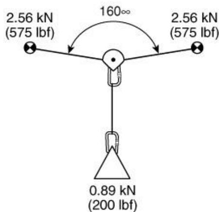
At 150 degrees, the load on each anchor would be 200%.
