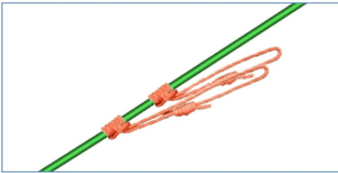
The tandem prusik belay is highly effective in arresting falls as well as decreasing the distance the load travels before coming to a stop.
