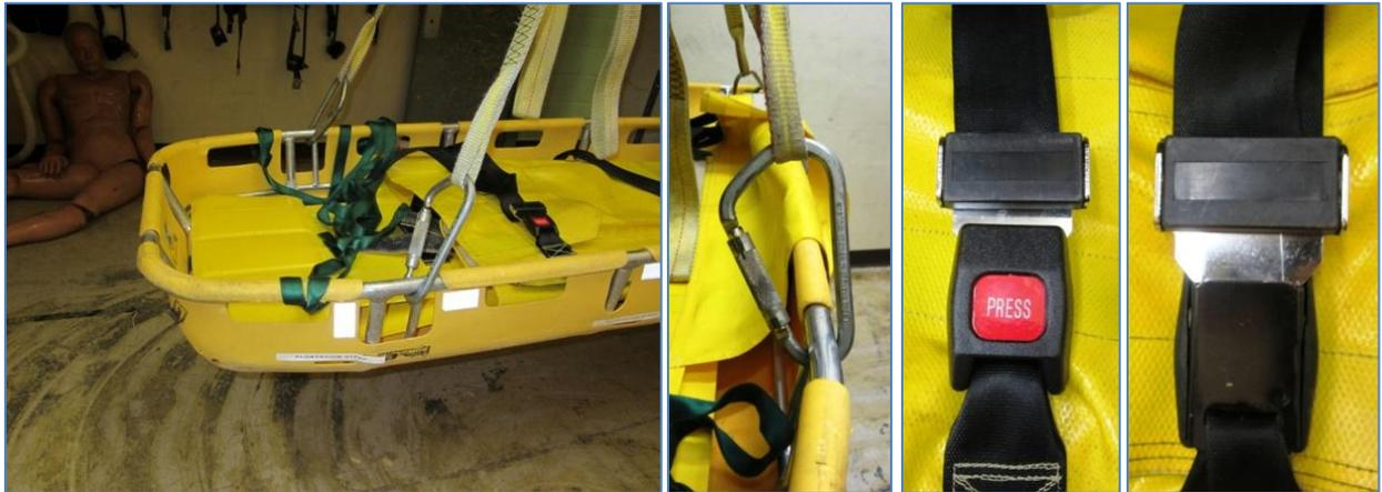
The basket's spider straps are rigged into a plate.
