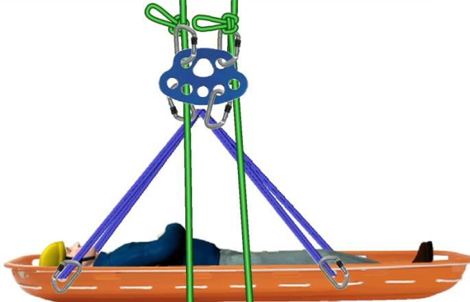
Prusik on each line allows for adjustment.
