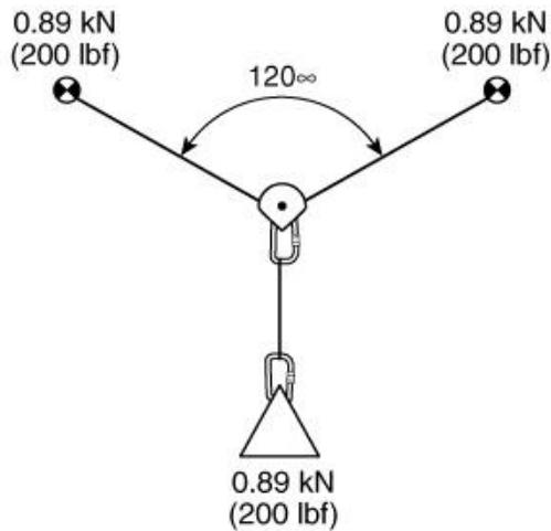
If the angle is increased to 120 degrees, 100% of the load will be imposed on each anchor.
