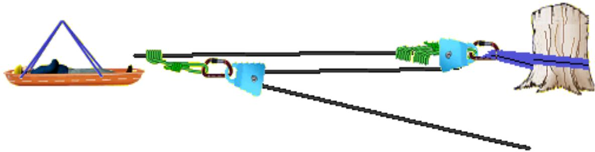
Remember a breaking device is required in the system. If the rescuers let go of the haul line gravity will take over.
