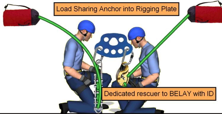
Load Sharing Anchor into Rigging Plate
