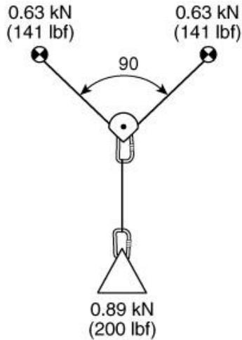
If the angle in the load-distributing anchor system is increased to 90 degrees, the resulting weight on each anchor is 71% of the load.
