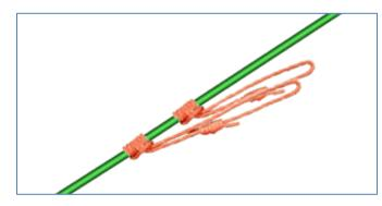
The tandem prusik belay is highly effective in arresting falls as well as decreasing the distance the load travels before coming to a stop.
