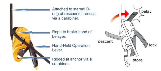
A dedicated belayer will use two hands while operating this device. One hand controls the lever while the second hand holds the braking side of the rope.
