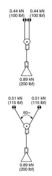
At a 0 degree angle, the load on each anchor will be 50%. With a two-point loaddistributing anchor system holding a load of 200 pounds, each anchor holds approximately 50% of the load, or 100 pounds.
