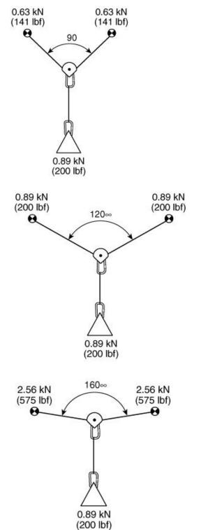
If the angle in the loaddistributing anchor system is increased to 90 degrees, the resulting weight on each anchor is 71% of the load.
