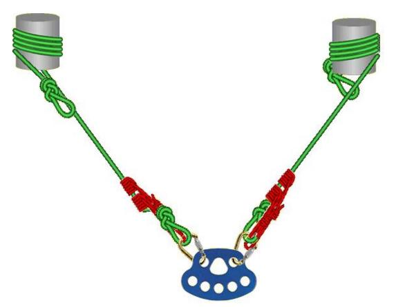
A tensionless-hitch captures each anchor. It's terminated by using a fig-8 followthru back to the rig line.
