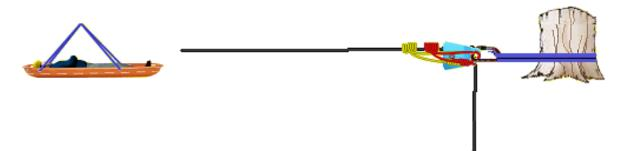
If the FIRST moving pulley in the system is at the LOAD, the system will be odd. This is a 3:1 Mechanical Advantage.
