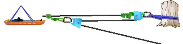
Remember a breaking device is required in the system. If the rescuers let go of the haul line gravity will take over.
