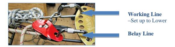
Any required *outside edge attendants* shall be placed onto a 2-rope system attached to an independent rope and anchor system from the basket.
