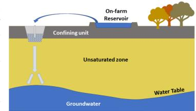
Fig. 2: Infiltration gallery conceptual drawing.
