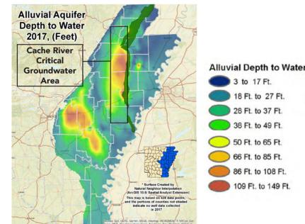
Fig. 1: MRVA aquifer cones of depression (ANRC, 2018).
