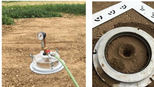
Fig. 1 Modified Mini-JET device (left), scour hole after the experiment (right)
