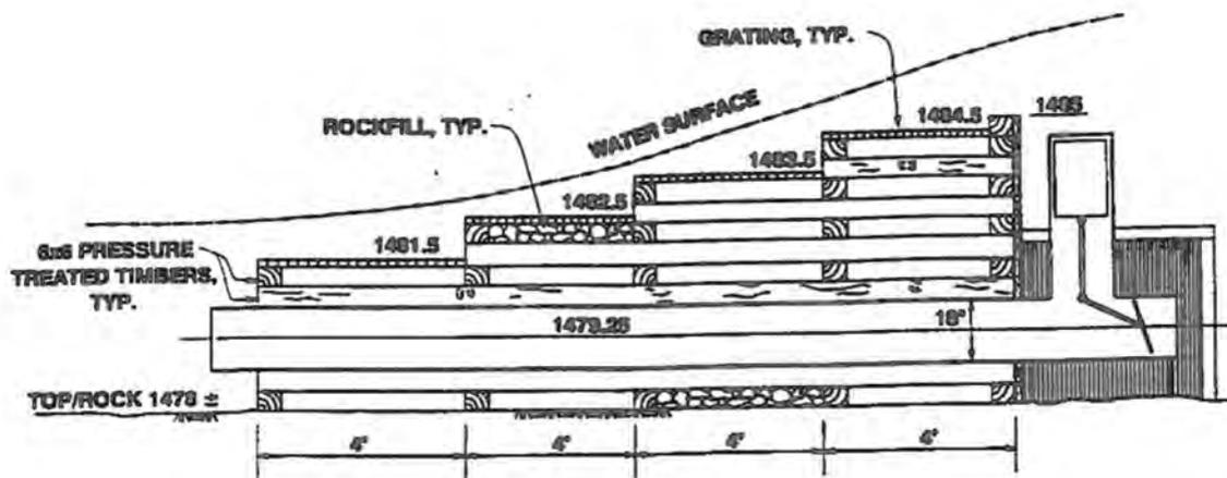
Fig. 1. Section view of timber crib weir.
