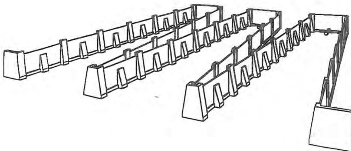
Fig. 2. Perspective view of three-bay labyrinth weir.
