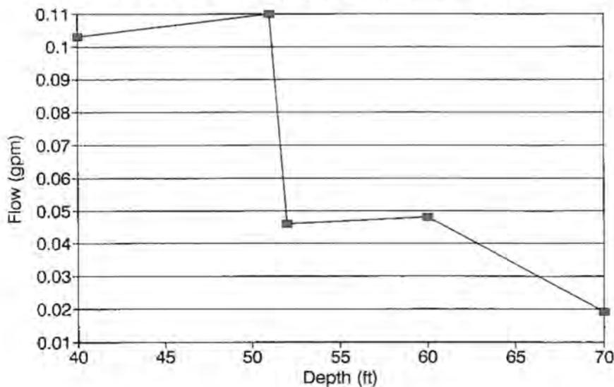
**Fig. 2.** Borehole flowmeter survey of corehole 2. A single flowing fracture was detected in this survey.
