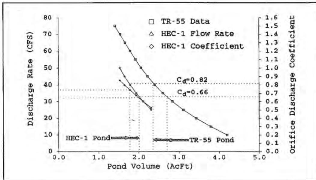
Fig. 2B. TR55 & HEC1 pond design comparison for assumed orifice discharge coefficients.
