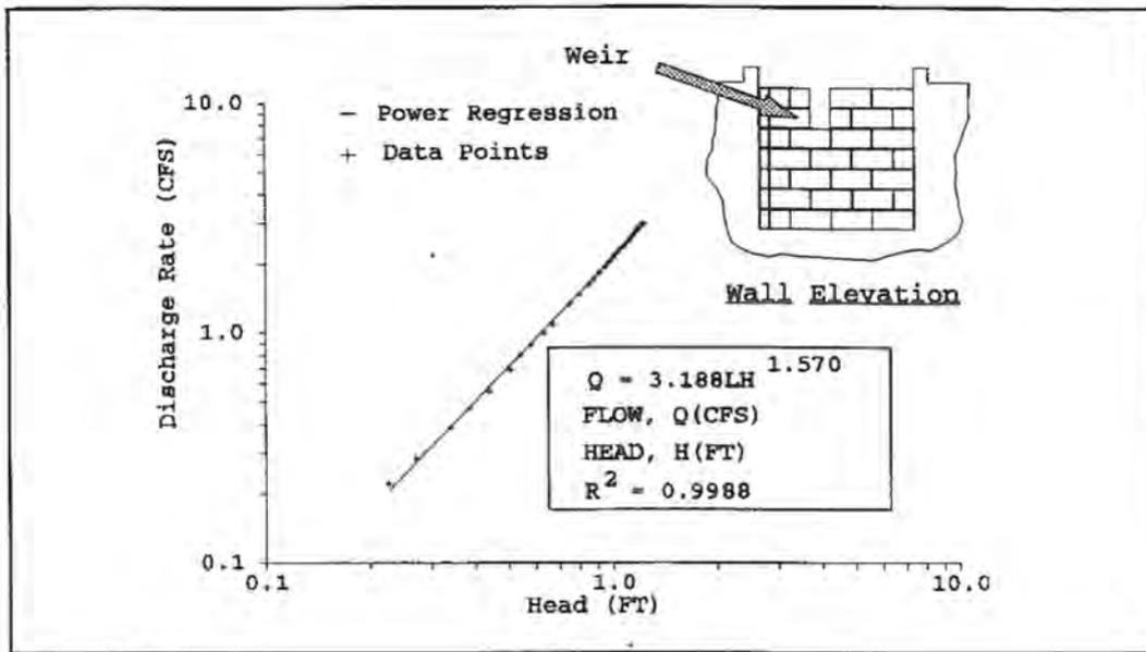
Fig. 2A. Discharge rating curve for 8" wide x 16" high weir only (Test 10).
