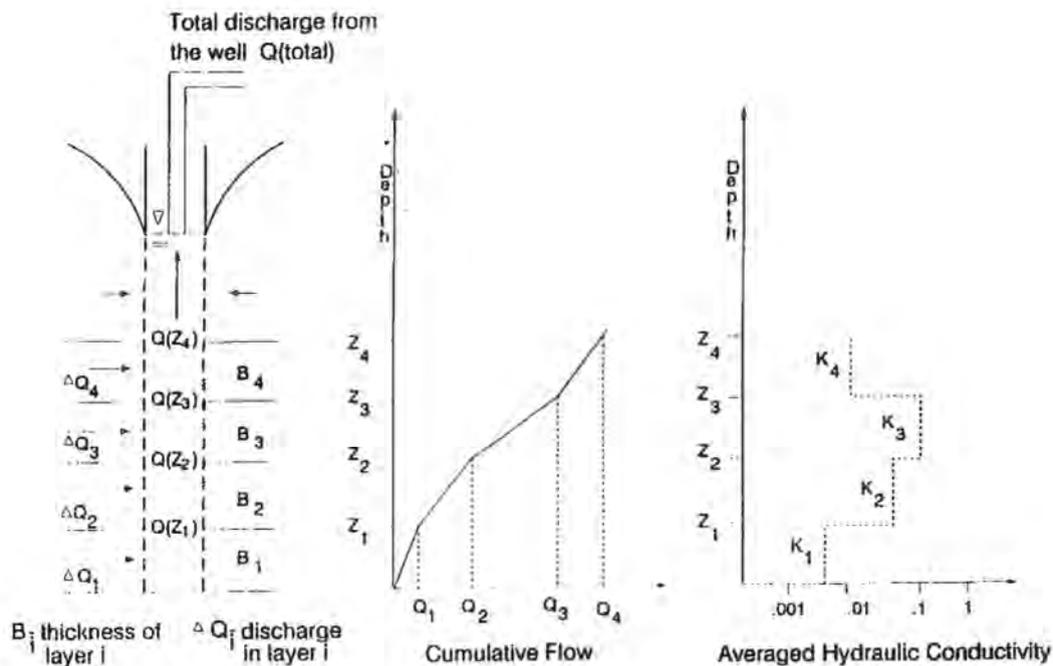
**Fig. 1. Schematic of Horizontal Flow to a Well and the Profiles of the Cumulative Flow and the Calculated Hydraulic Conductivities.**
