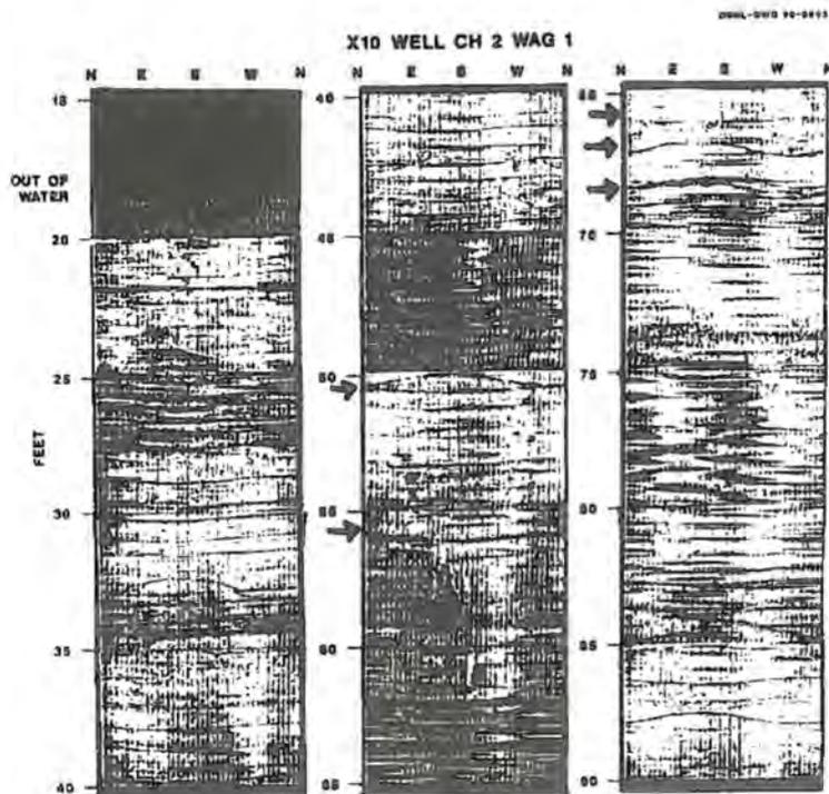
**Fig. 3.** Borehole televiewer log of corehole 2. Sinusoidal patterns are indicative of fractures (arrows).
