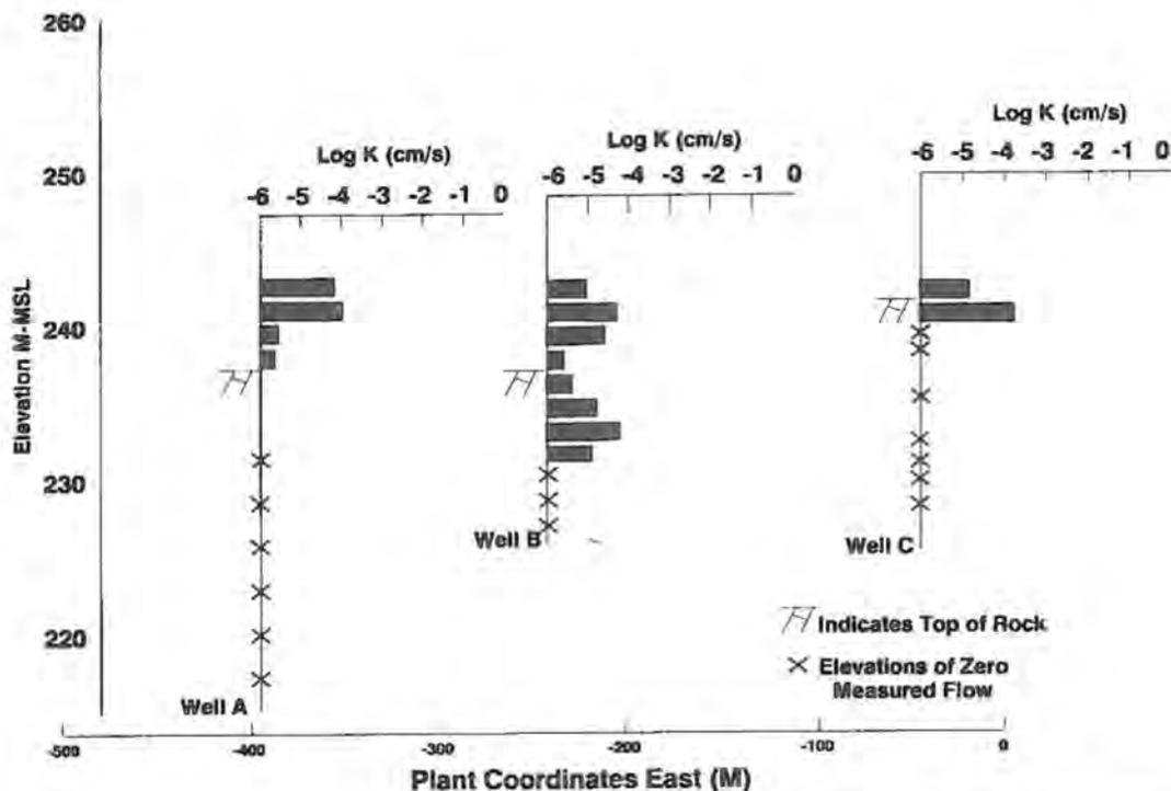
Fig. 2. Bull Run borehole flowmeter results. CROSS SECTION - 1847 North. Tested December 1990.
