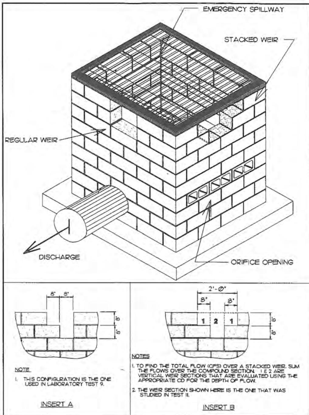
Fig. 1. Typical concrete block discharge structure.
