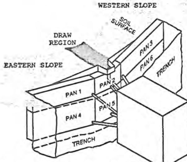
Fig. 1. Schematic of stainless-steel pans placed against trench face for collecting subsurface flows from the subcatchment.
