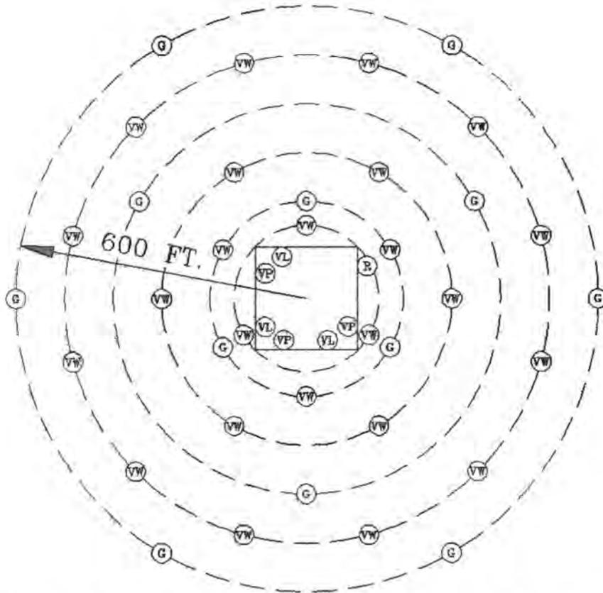
**Figure 1:** Locations of shallow vadose-zone wells (VW), ground water wells (G), vadose-zone lysimeters (VL), vadose-zone pans (VP), and runoff flume (R) around one acre field test plot.
