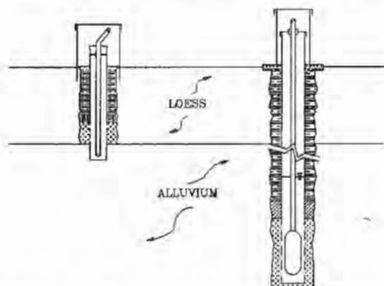
Figure 2: Cross-section of ground water and perched water sampling wells.
