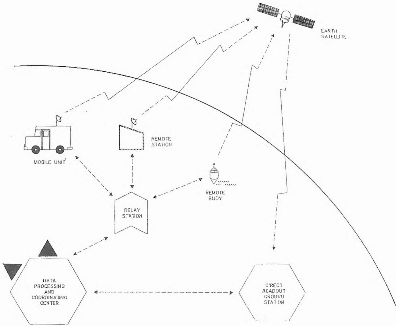
Figure 1. Proposed regional network using portable aquatic automated biomonitoring systems
