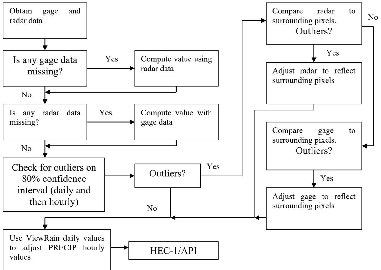
Figure 2 – Flow chart for error reduction procedure
