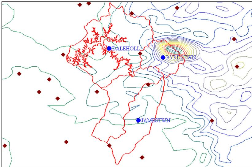
Figure 1 – ViewRain image of Dale Hollow Basin with radar data from May 24 – June 24, 1997 storm event.
