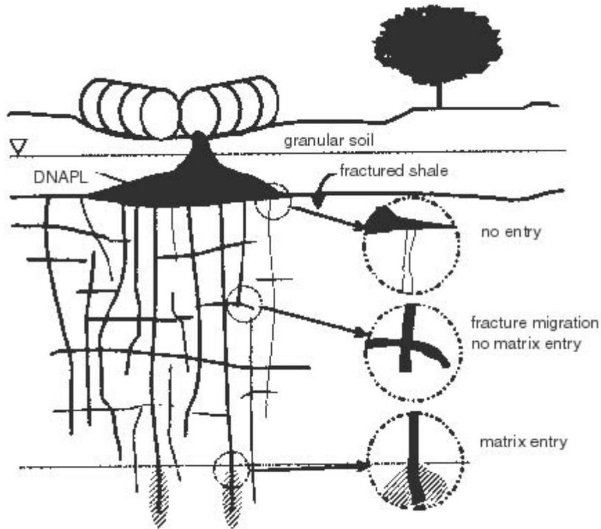
Figure 1. Immiscible DNAPL entry into fractures and matrix is illustrated. At the top inset, capillary pressure is insufficient for fracture entry. At the middle inset, capillary pressure is sufficient for fracture entry, but not matrix entry. At the bottom inset, capillary pressure exceeds matrix entry pressure and immiscible phase DNAPL can enter the porous matrix. (Adapted from Cropper, 1998).
