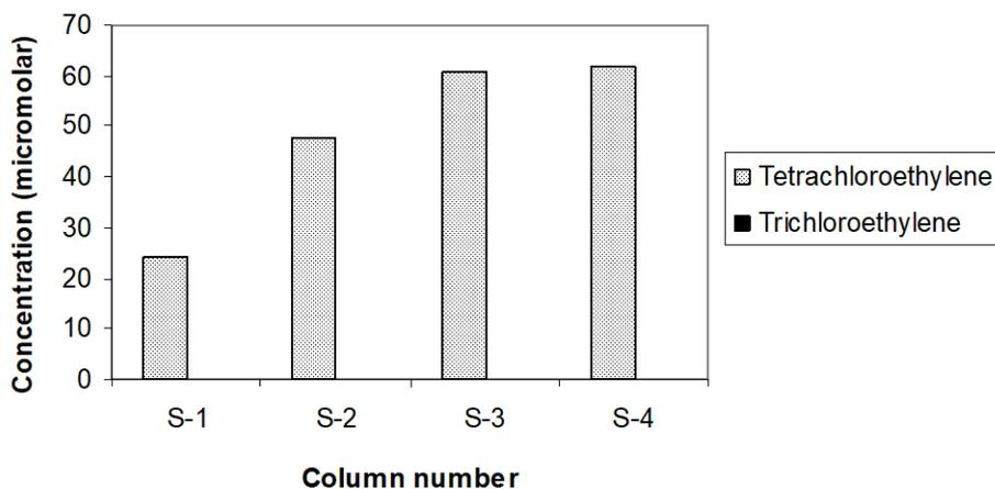
Figure 2. Tetrachloroethylene (PCE) extracted from small columns containing PCE dissolved in water. Trichloroethylene (TCE) was not detected in any treatment. Column 1 had PCE, Direct current (DC), and vitamin B12. Column 2 had PCE and a DC. Column 3 had PCE and vitamin B12. Column 4 had PCE and no vitamin B12 or DC. The coefficient of variation was 6, 10, 23 and 13 percent respectively.
