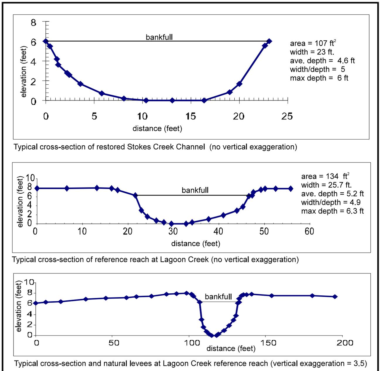
Figure 2: Typical cross-sections of Stokes Creek restored channel and reference reach
