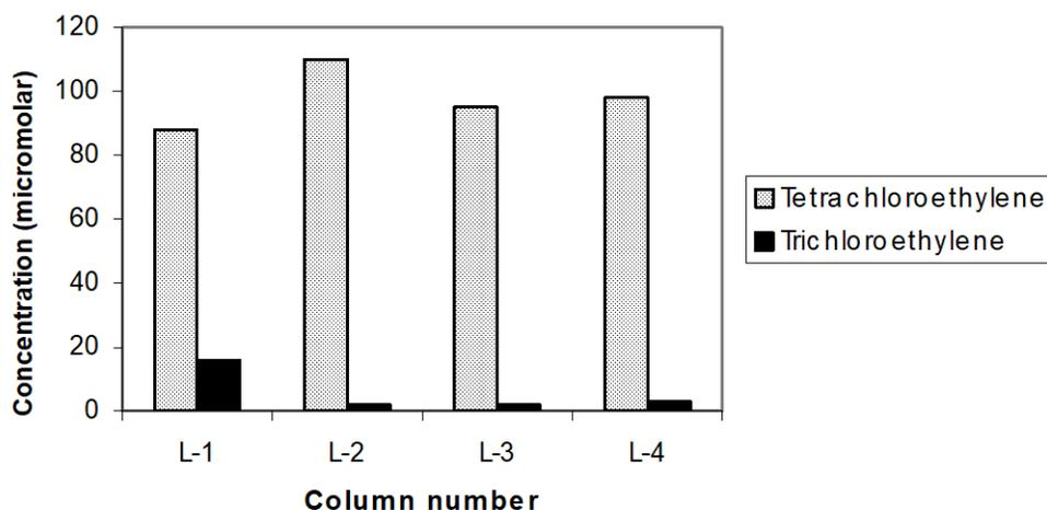
Figure 1. Remaining PCE and TCE extracted from the soil columns after 7 days of treatment. Column 1 had PCE, 200 mV DC, and B12. Column 2 had PCE and B12. Column 3 had PCE and 200 mV DC. Column 4 had PCE and no B12 or DC.
