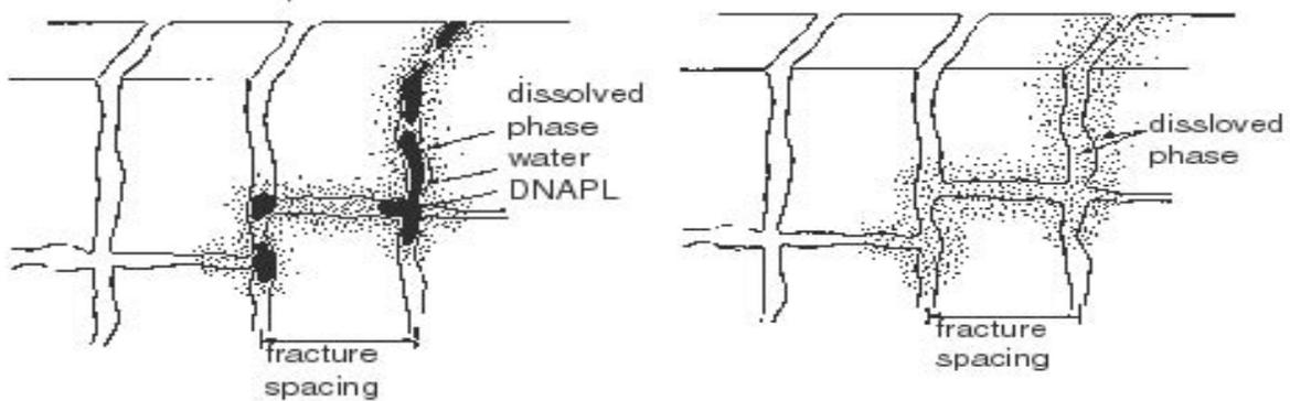
Figure 2. Effects of dissolution and matrix diffusion is illustrated. On the left, the processes contribute to disconnect columns of DNAPL. On the right, pure phase DNAPL has disappeared leaving "haloes" of dissolved phase in the matrix adjacent to the fracture. (Adapted from Parker et al., 1996).
