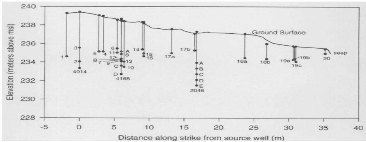
Figure 1: Cross-section of wells at the WAG-5 site showing the location and sampling depths of all groundwater monitoring wells (Jardine, 1997).
