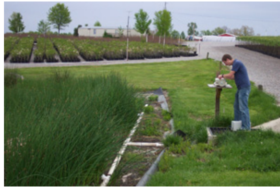
Illustration 2. Checking the Stevens chart recorder
