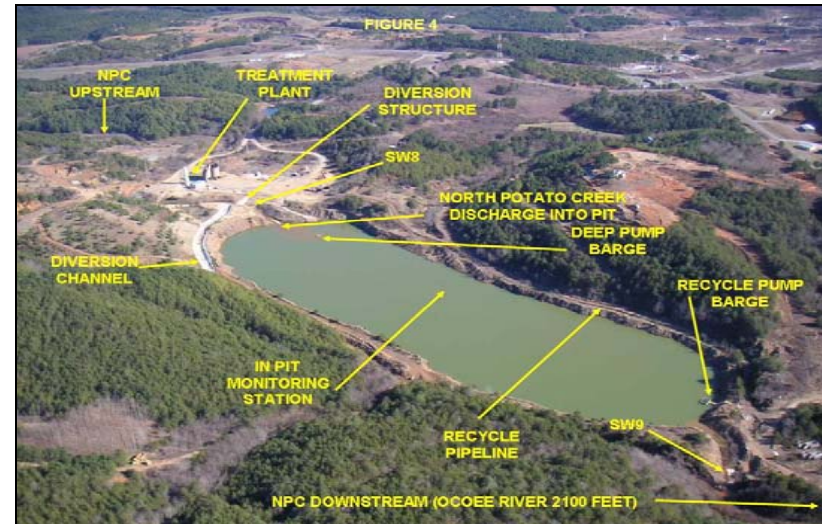
Figure 4. SMP Monitoring Locations
