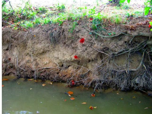
**Figure 3. Spray-painted erosion pins on banks of Nails Creek (left) and Ellejoy Creek (right).**
