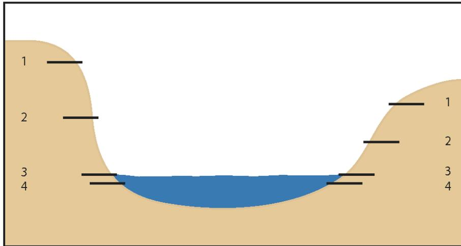
**Figure 2. Diagram of arrangement of erosion pins at a cross-section.**
