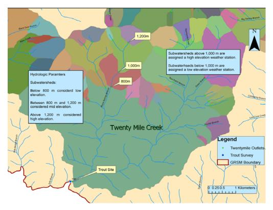
Figure 1. HSPF parameterization.
