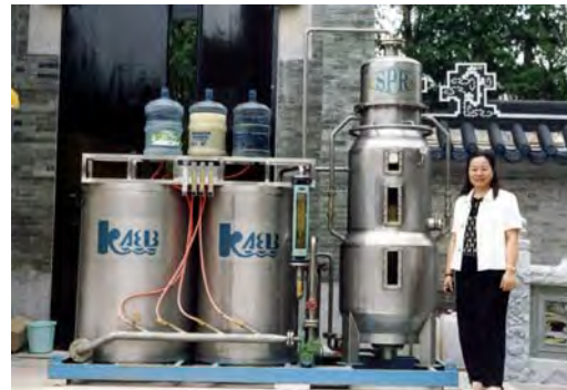
Figure 21. SPR system to treat Municipal Sewage into Recycled Water. (CA. USA)
