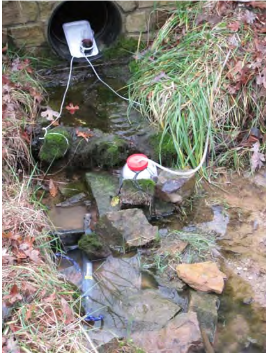
Figure 3: Photograph showing the dye and salt release mechanism. Also shown in the picture are the 1 st flush sampler and the YSI datasonde.
