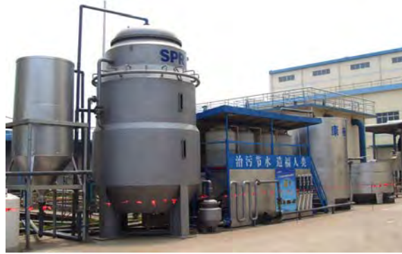
Figure 18. 600cum/d SPR-30 system (CHINA)
