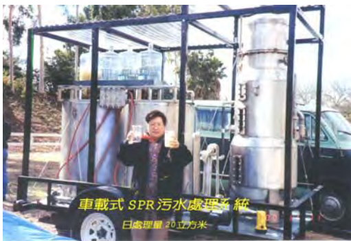
Figure 21. SPR system to treat Municipal Sewage into Recycled Water. (CA. USA)
