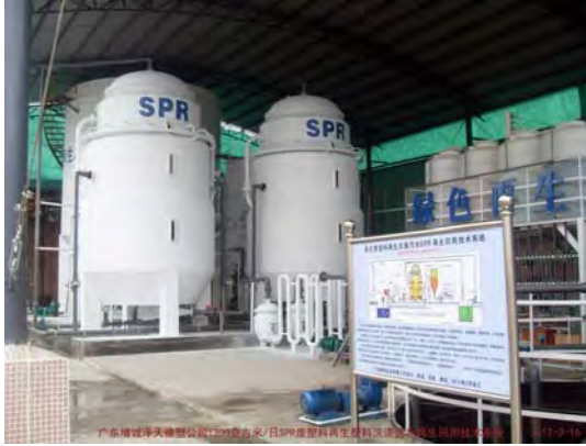
Figure 20. SPR System for 1200cum/day on plastics recycling industry. (2012.2 & 2012.3 CHINA)
