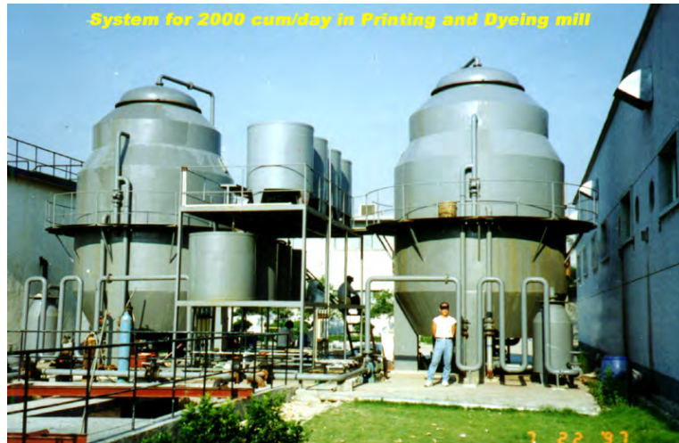
Figure 13. SPR to treat the wastewater from the printing and dyeing mill for reuse. (HongKong)
