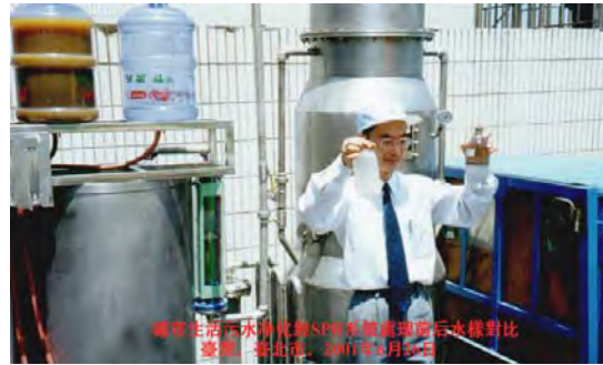
Figure 15. SPR System for reusing of municipal effluents for communities in city. (Taiwan)
