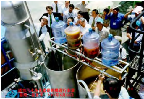
Figure 15. SPR System for reusing of municipal effluents for communities in city. (Taiwan)
