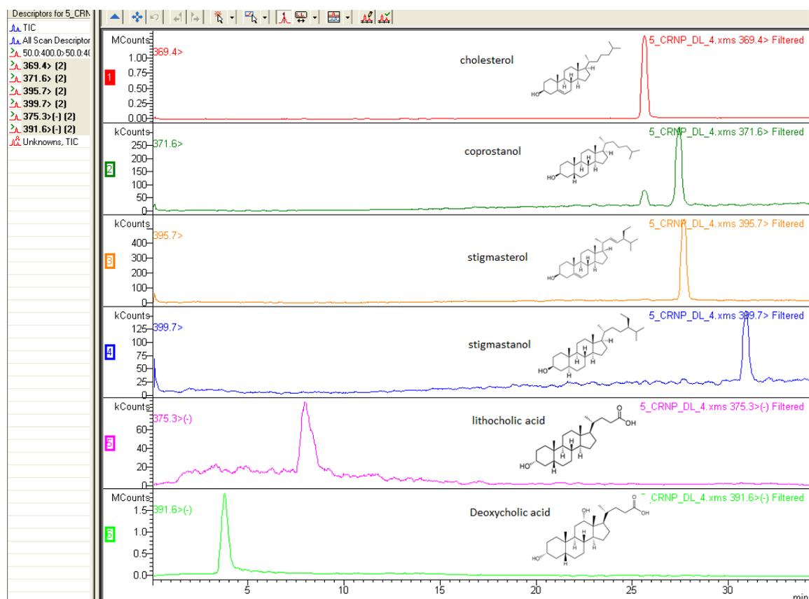
Figure 1. Chromatographic separation of bile acids and fecal sterols using Zorbax Eclipse XDB-C8 (3.0 × 150 mm × 3.5µm) column.
