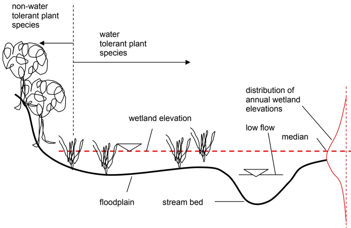
Figure 1. Section of Stream and Floodplain
