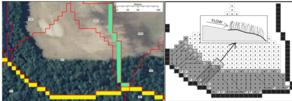
Figure 1. Schematic of GIS technology for the estimation of riparian vegetation sediment trapping efficiency at a watershed scale. Individual concentrated flow paths are represented as one-dimensional profiles into STE models. A weighted average of all flow path profiles generates a representative trapping efficiency value for each AnnAGNPS cell in the watershed.
