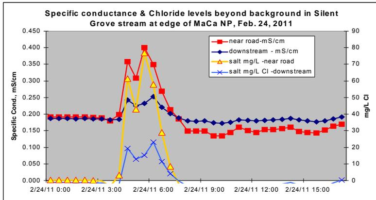
Figure 2. The conductivity and estimated chloride levels in Silent Grove sinking stream following a road salting in February, 2011. The upstream station is 50-feet from the road, and the downstream station is ~500 feet downstream, near the sink.
