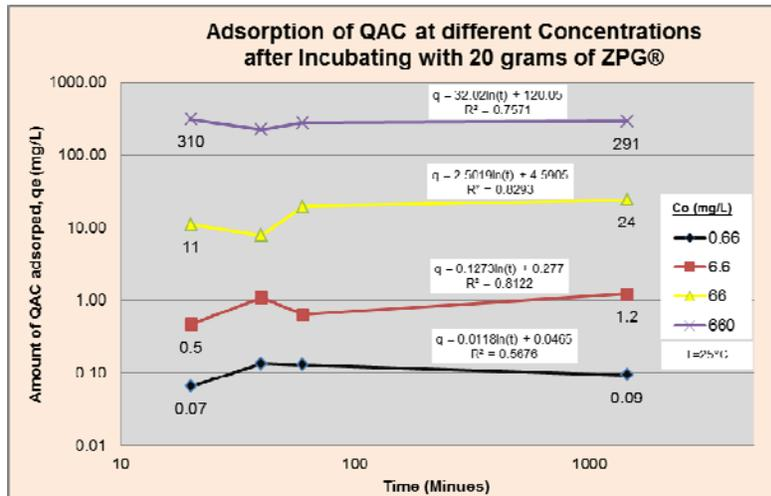
Figure 7. The amount of QAC adsorbed over time with different concentrations was compared. The process is best described by natural logarithm which means the rate of change of QAC adsorbed decreases over time. Also, the adsorption rate is higher with higher initial concentration. The difference in adsorption rate is due to the diffusion effect. The higher concentration of QAC has higher possibility to be adsorbed onto the filter media.
