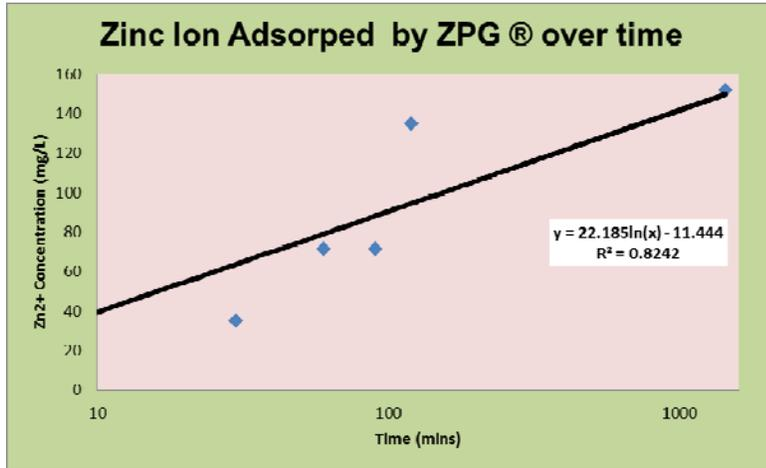
Figure 5. Initial concentration of 227mg/L of Zinc ion is used to determine the amount of  $\text{Zn}^{2+}$  adsorbed to ZPG®. The nature logarithm curve indicates that the adsorption rate decreases over time,  $dq/dt = 22.19/t$ .
