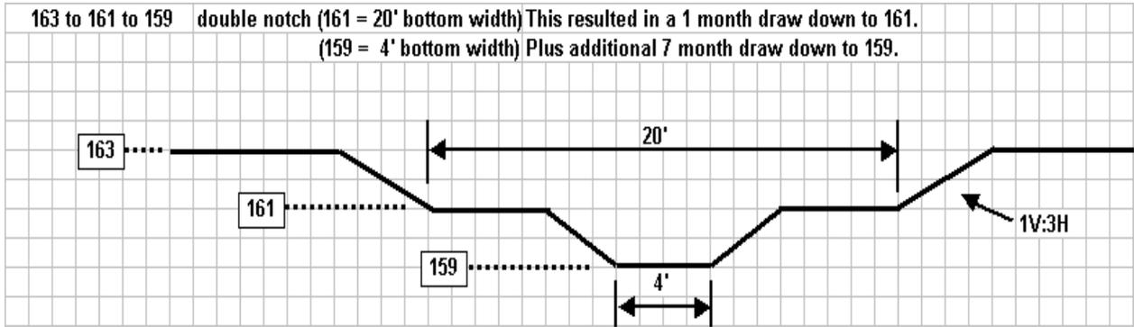
Figure 2. Section Through Crest of Riprap Weir
