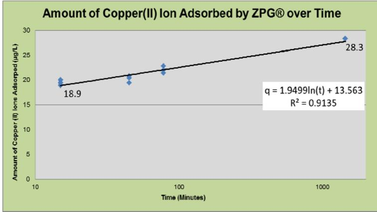
Figure 2. Initial concentration of  $40\mu\text{g/L}$  of Copper(II) ion is used to determine the amount of  $\text{Cu}^{2+}$  adsorbed to  $\text{ZPG}^{\text{®}}$ . The nature logarithm curve indicates that the adsorption rate decreases over time,  $dq/dt = 1.95/t$ .
