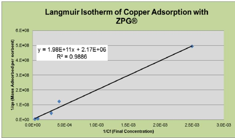
Figure 3. Langmuir isotherm is found to best describe the  $\text{Cu}^{2+}$  adsorption process onto  $\text{ZPG}^{\text{®}}$ , Physisorption and chemisorption are both expected to contribute in the treatment process. Equilibrium concentration of  $\text{Cu}^{2+}$  in solution,  $C_e$ , is  $4.61\mu\text{g/L}$ . The adsorption capacity of  $\text{ZPG}^{\text{®}}$ ,  $K_d$  is  $11\mu\text{g/g}$ .
