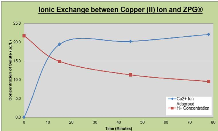
Figure 4. Langmuir isotherms indicate that chemisorption occurs, ionic exchange is expected between the dissolved Cu ion and sodium ion in zeolite. The exchange process can be determined by the change in pH value. An increase in pH value is found during the adsorption process. It agrees with the assumption that ionic exchange occurs. The increase in pH is due to the dissolution of sodium ion
