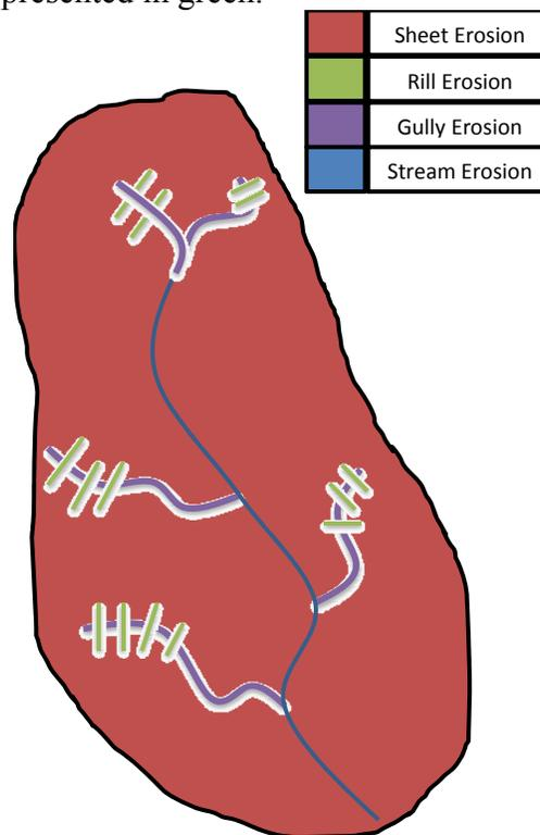
Figure 8. Synthetic Watershed Indicating Erosional Sources
