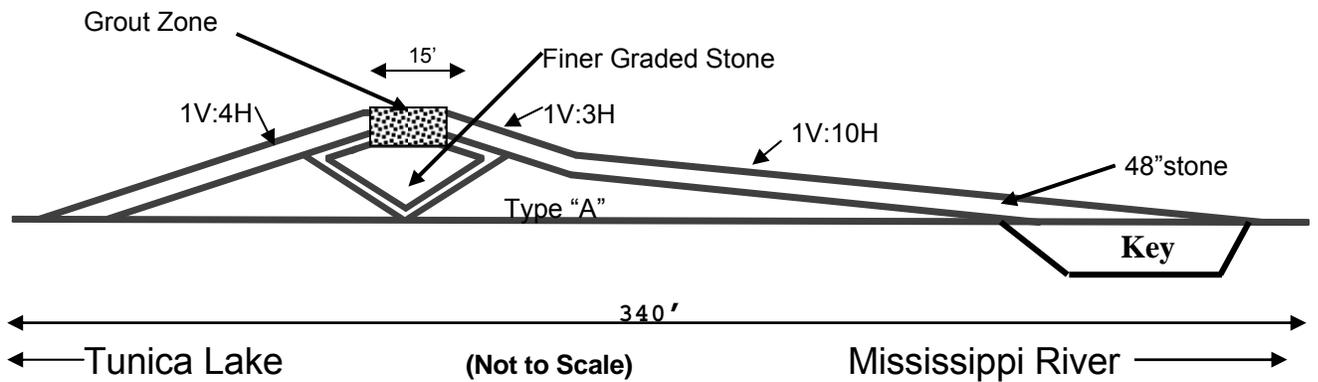
Figure 3. Profile Centerline of Riprap Weir
