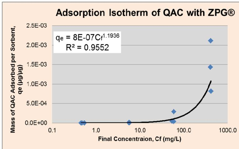
Figure 6. Freundlich isotherm is found to best describe the QAC adsorption process onto ZPG®. Chemisorption is negligible because QAC does not dissolve in water, and no ionic exchanged is expected. Physisorption is expected to be the major contributing process in treatment. Granular Activated Carbon and Perlite are the major contributors in the adsorption process. The adsorption capacity of QAC onto ZPG®,  $K_d$  is  $0.8\mu\text{g}/\text{g}$ .
