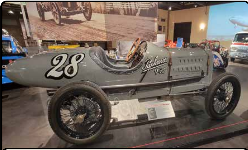
1911 Packard - 424 Cu. In. V-12 - 88 HP
