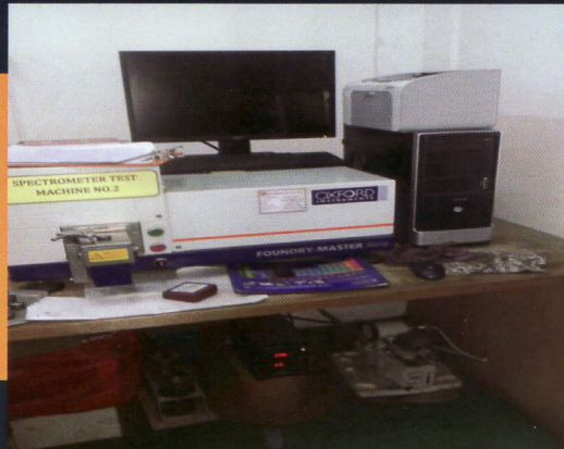
Testing chemical composition of Molten steel and billets equipment
