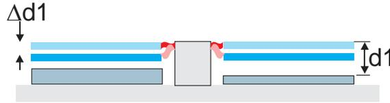
Figure 4. Schematic diagram of the cross section of two mirror elements in the FP array showing the quiescent gap between the top and bottom mirrors  $d_1$  and the tuning range  $\Delta d_1$
