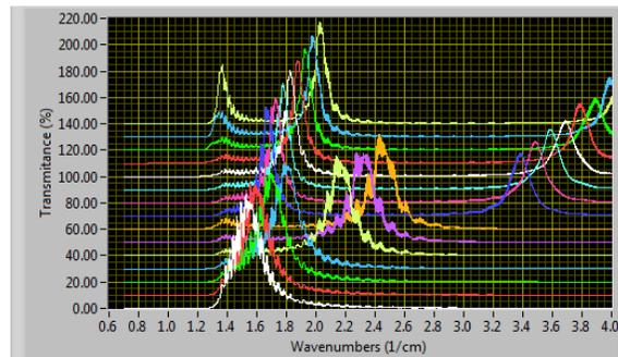
Figure 8. Shows the damping of the Si-Air effect by using an A/R coating.
