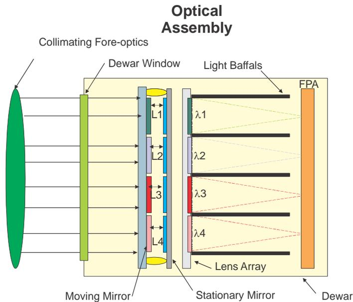
Figure 1. Schematic of the optical components in the test fixture for the FPTF.
