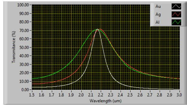
Figure 6. Shows the transmission peaks for Au, Ag, and Al at 2.15 microns.
