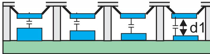
Figure 3. Schematic diagram of the cross section of the FP array showing the quiescent gap determined by the thickness of the stationary mirror on the bottom.
