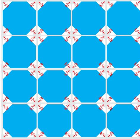
Figure 2. Schematic of the 4 x 4 Fabry-Perot tunable filter array.
