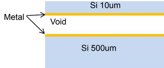
Figure 5. Schematic structure of the Fabry Perot cavity.
