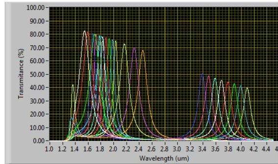
Figure 7. Transmittance summary for the 16 FP tunable filters, transmission through the Au film is falling as the wavelength increases. Higher order show up at lower wavelengths
