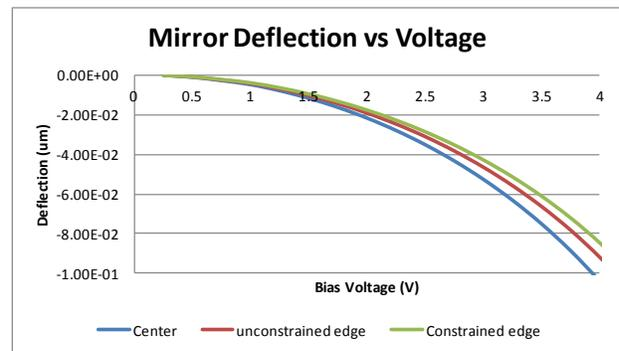
Figure 9. Shows the results for a 4 position constrained mirror with a weaker spring.
